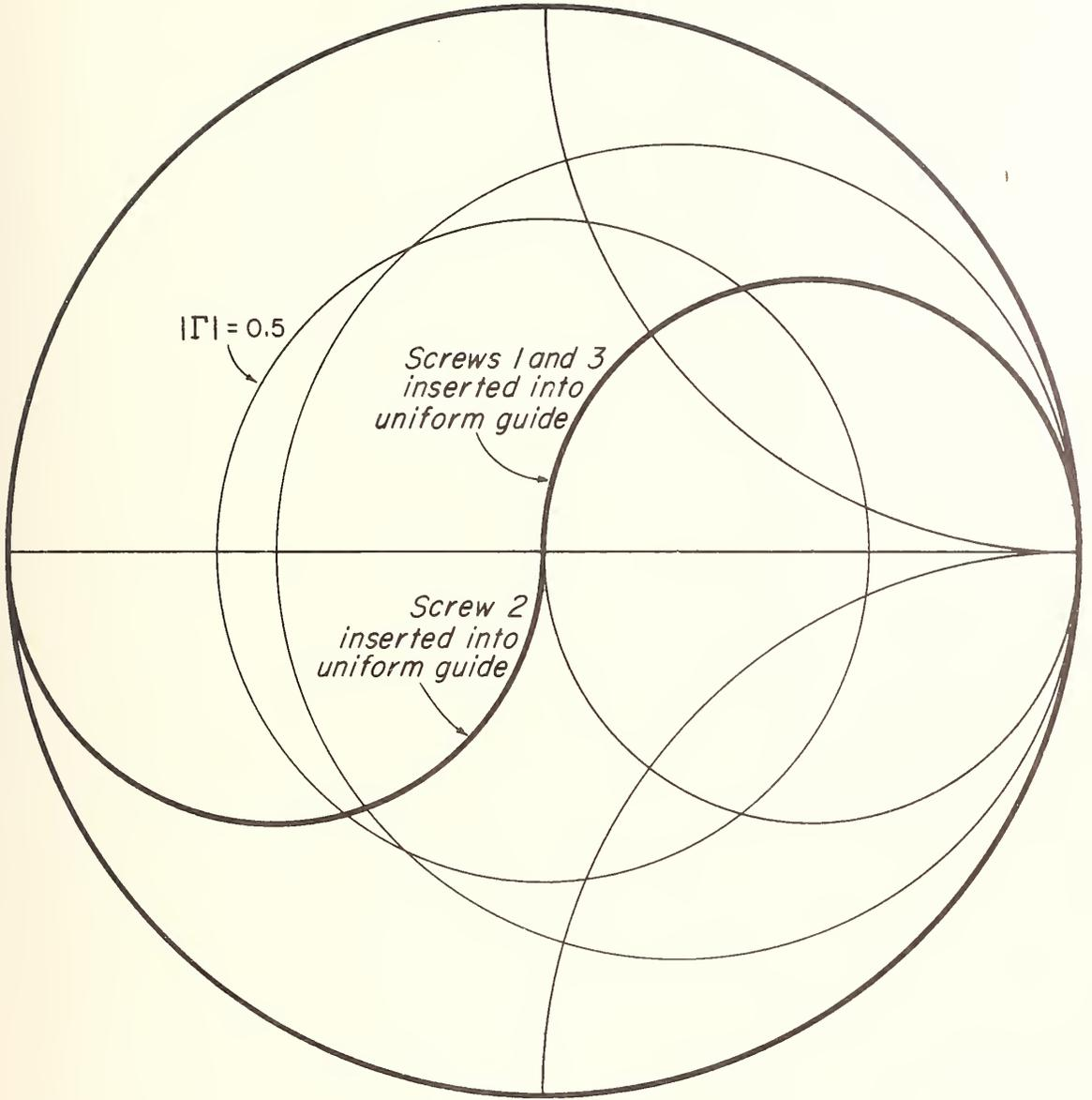
Figure 3. Normalized Smith admittance chart representation of the tuning capabilities of 3 screws spaced one-fourth guide wavelength apart.
