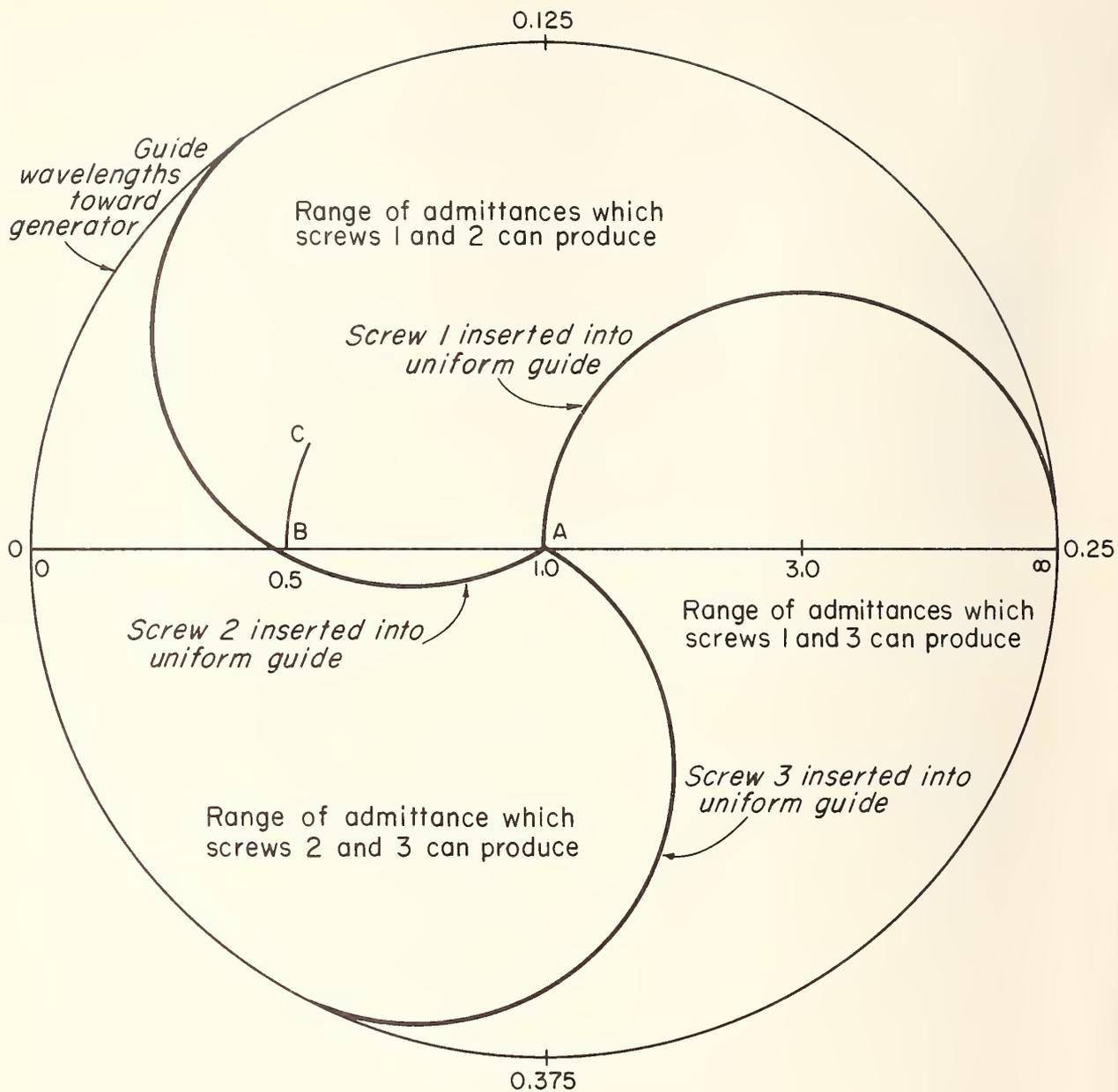
Figure 2. Normalized Smith admittance chart representation of the tuning capabilities of 3 screws spaced one-sixth guide wavelength apart at design frequency and reference plane at 1st screw.
