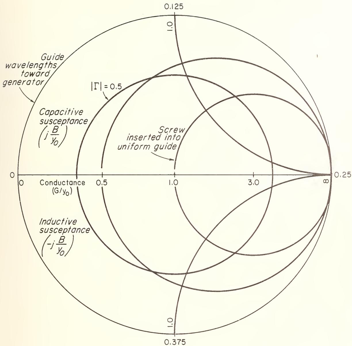
Figure 1. Normalized Smith admittance chart representation of a screw in a uniform waveguide.
