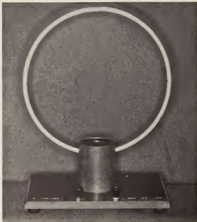
Figure 5.7. Standard Receiving Loop Used at 10 MHz.
