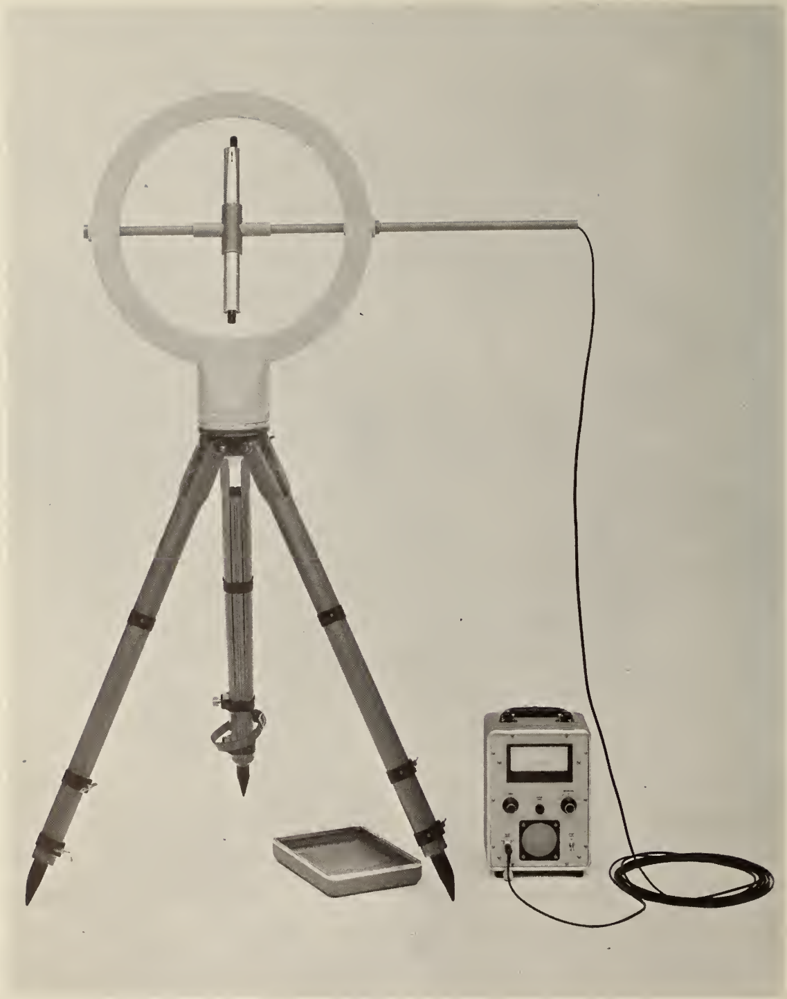
FIG. 19 THE COMPLETE NEAR-ZONE FIELD-STRENGTH METER
