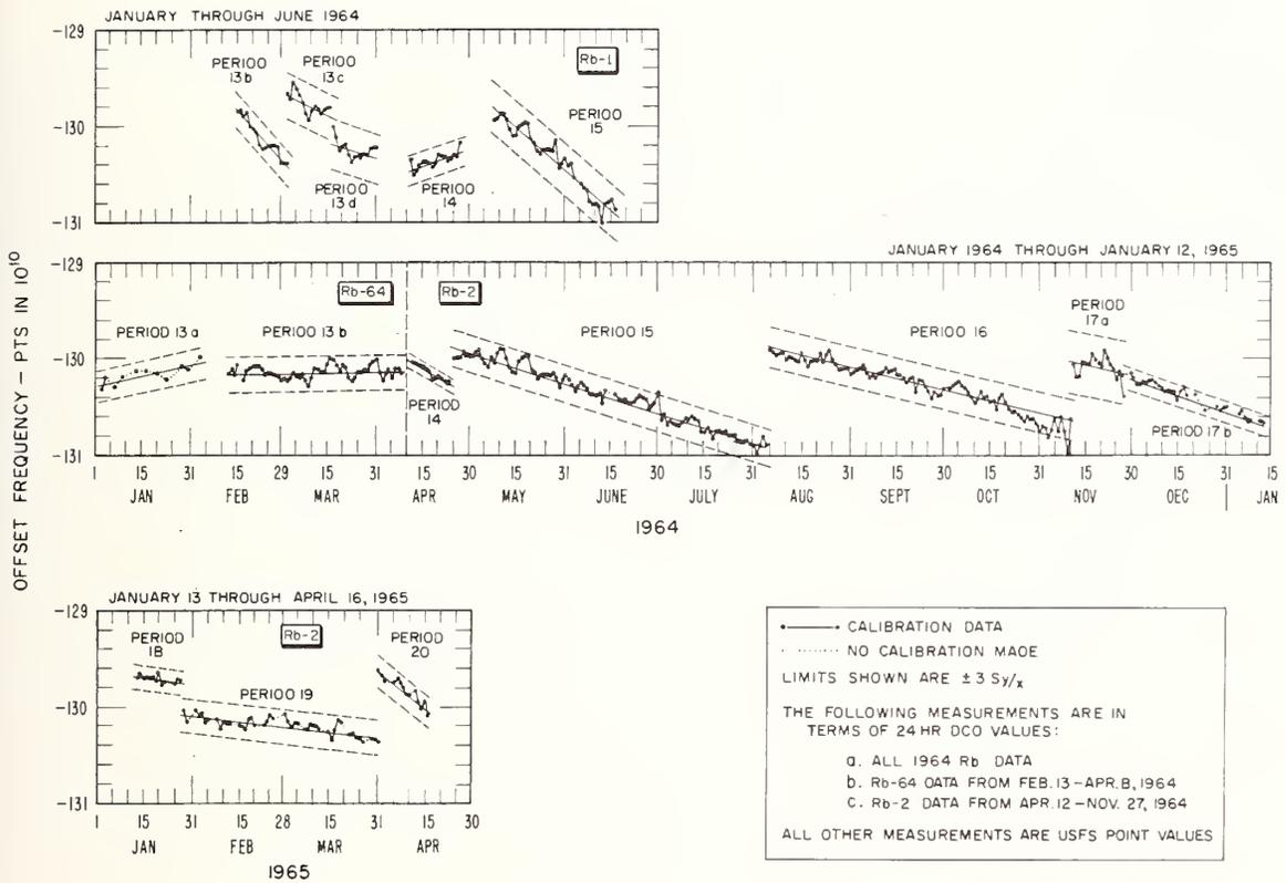
FIG. 3 CALIBRATION DATA OF Rb-1 AND Rb-2 DURING 1964 TO EARLY 1965 (Rb-64 DATA GIVEN IN PERIOD 13)
