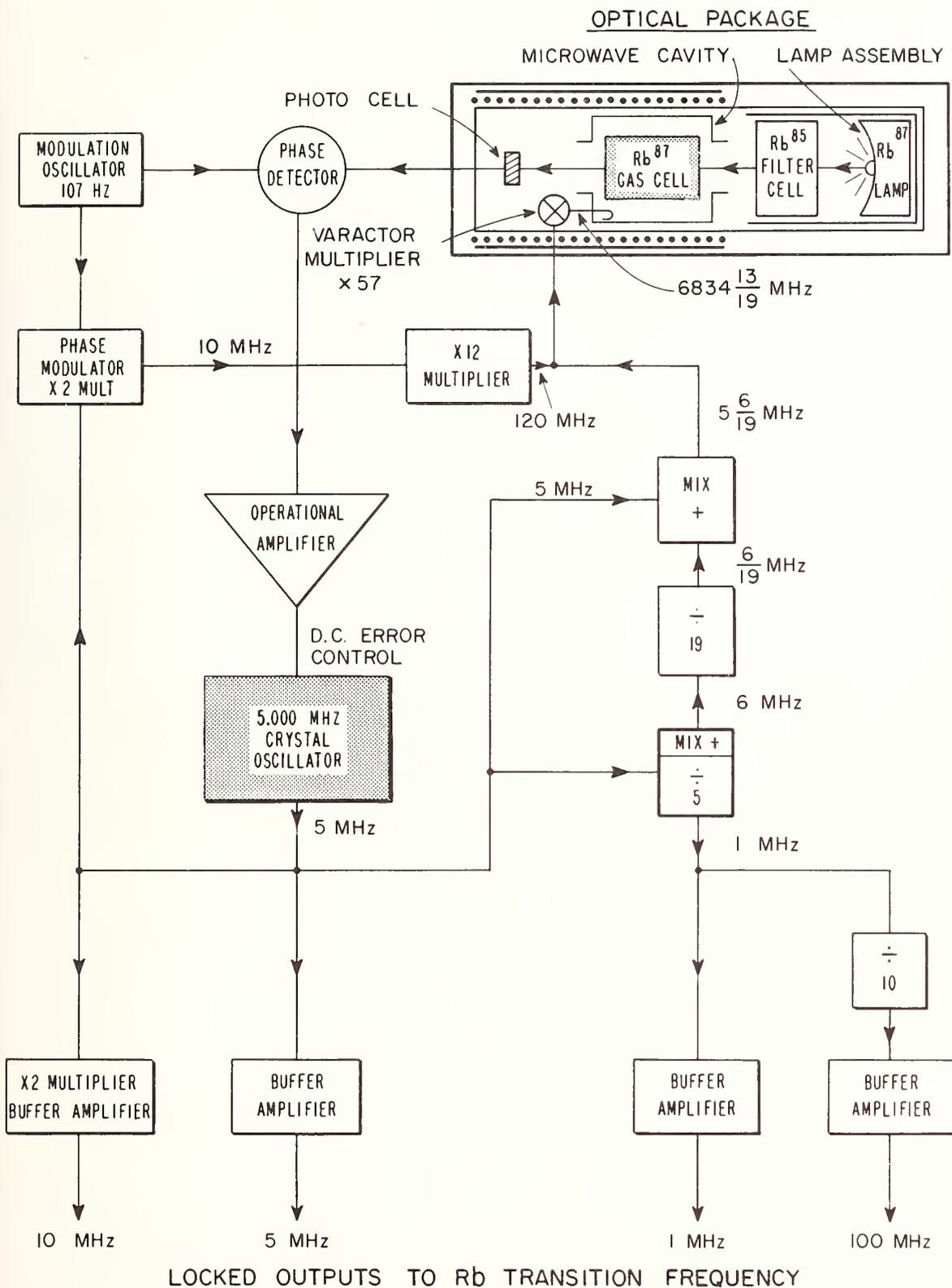
FIG. 1 BASIC SYSTEM OF Rb ATOMIC FREQUENCY STANDARD
