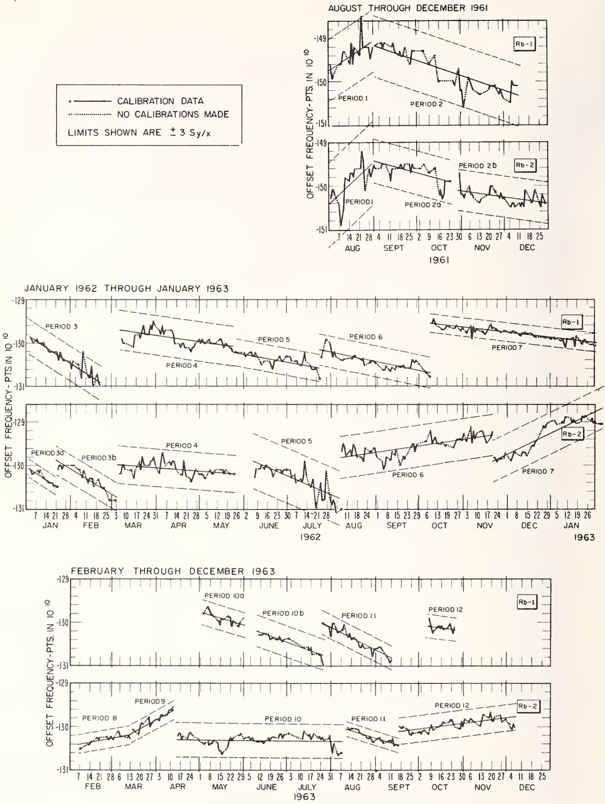
FIG. 2 CALIBRATION DATA OF Rb-1 AND Rb-2
