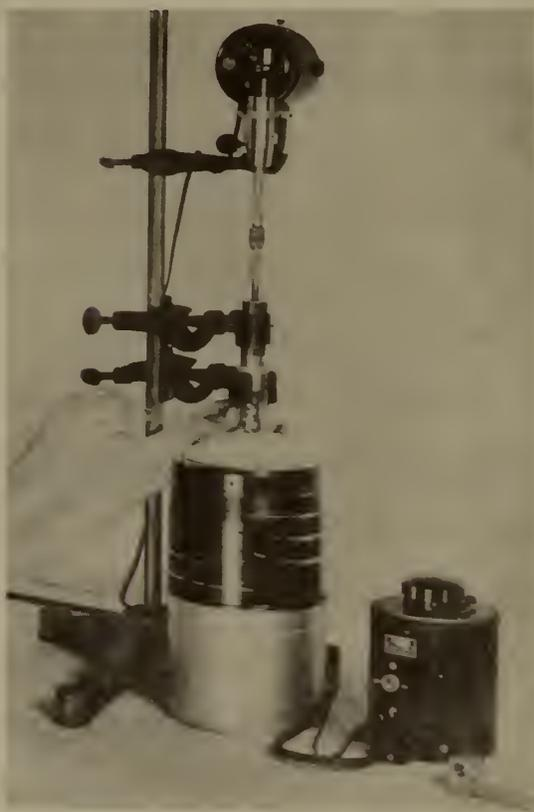
Figure 11. Apparatus for reduction of aldonic lactones.
