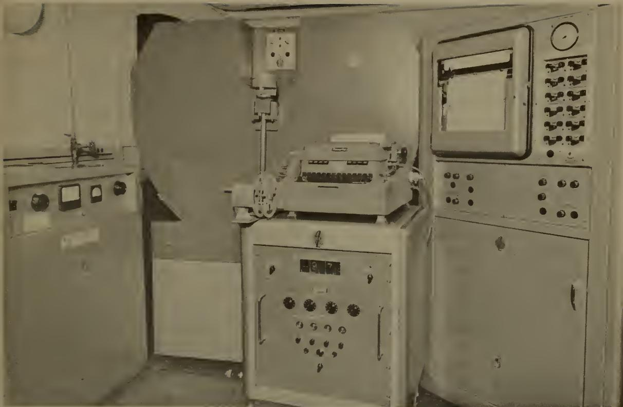
Figure 11. Multi-channel x-ray spectrometer. Left, x-ray tube power supply; center rear, spectrometer proper; right, signal integrating and conditioning console; center front, digital converter, programmer, and typewriter read-out with tape punch.
