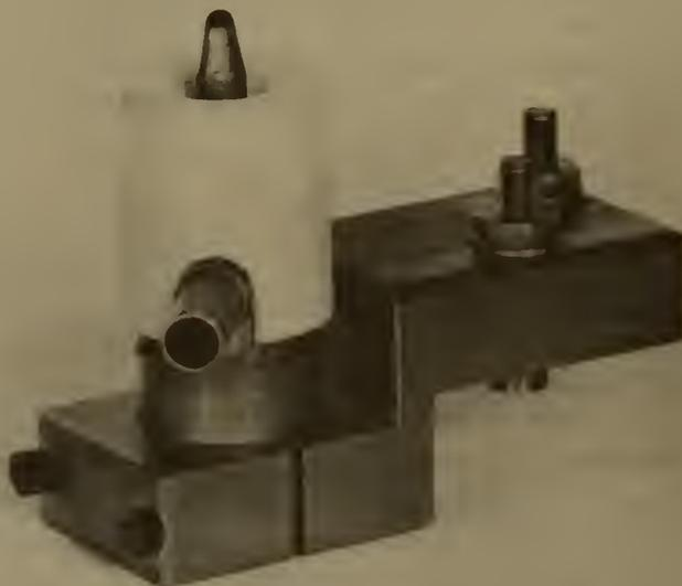
Figure 2. Device used for atmosphere control in inert-gas spark excitation.
