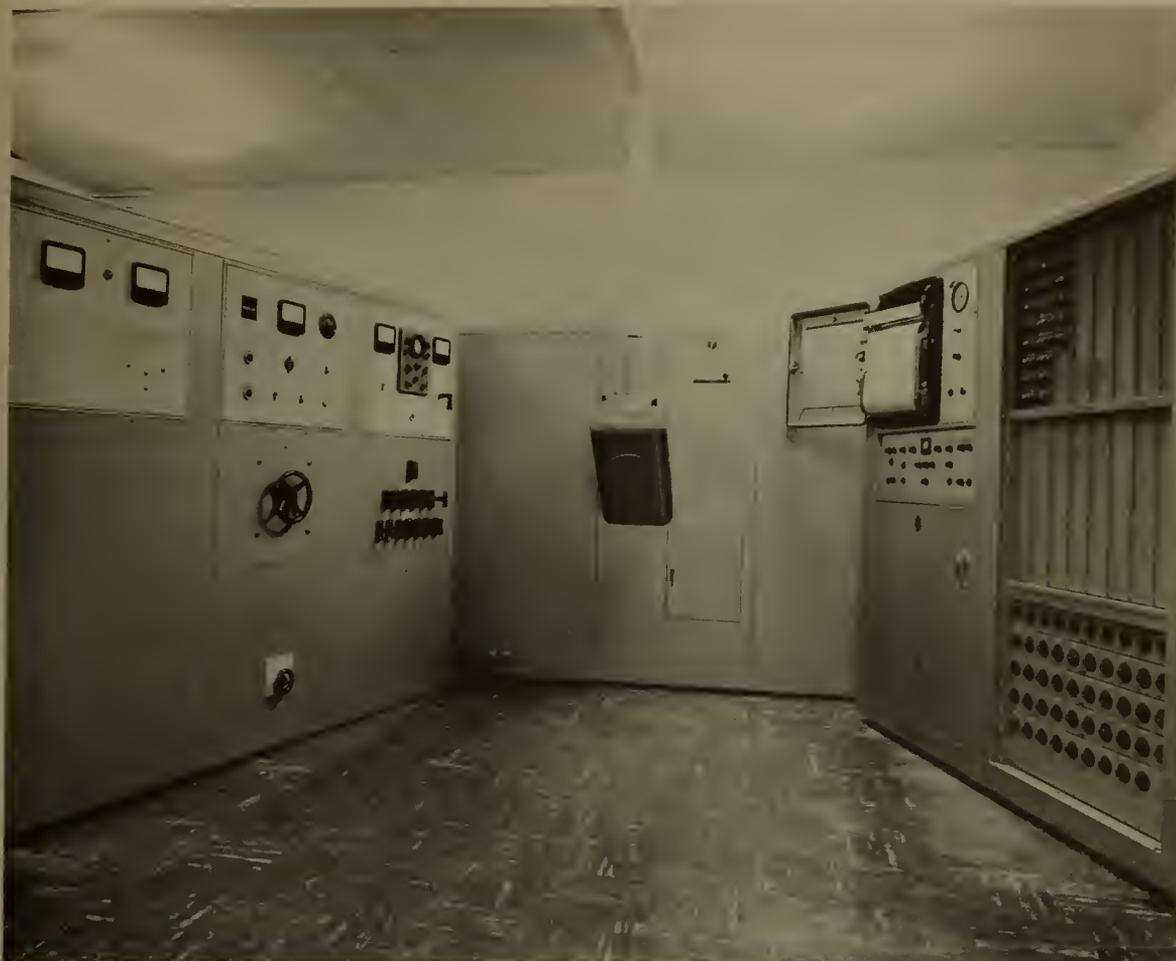
Figure 23. Multi-channel optical spectrometer. At left, excitation source console; center, 2-meter grating spectrometer with spark stand in front; right, recording console with chart recorder controls, and array of spectral line integrators.
