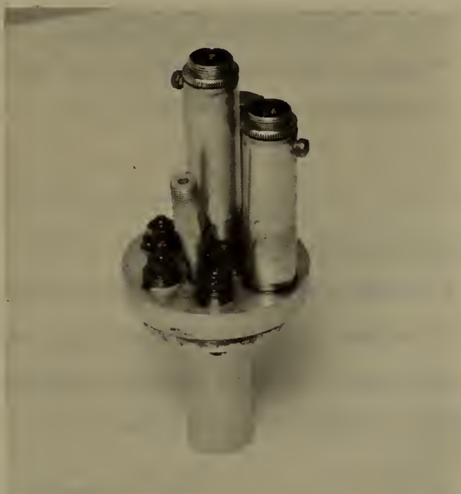
Figure 15. Three-terminal cell for measurements of dielectric constants.
