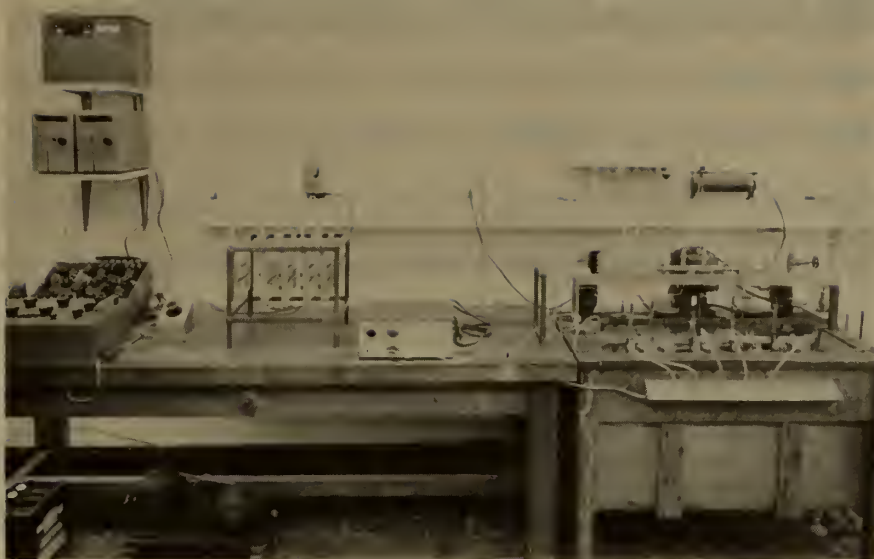
Figure 1. Equipment for the precise electromotive-force measurements on which pH standards are based.
