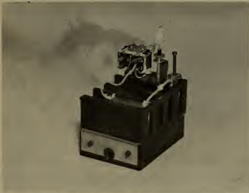
Figure 10. Controlled-temperature cell block for spectrophotometric measurements.
