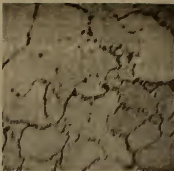
Figure 56. Electron Back-scattering Image of Platinum-13% Rhodium Working Standard, x 440.
