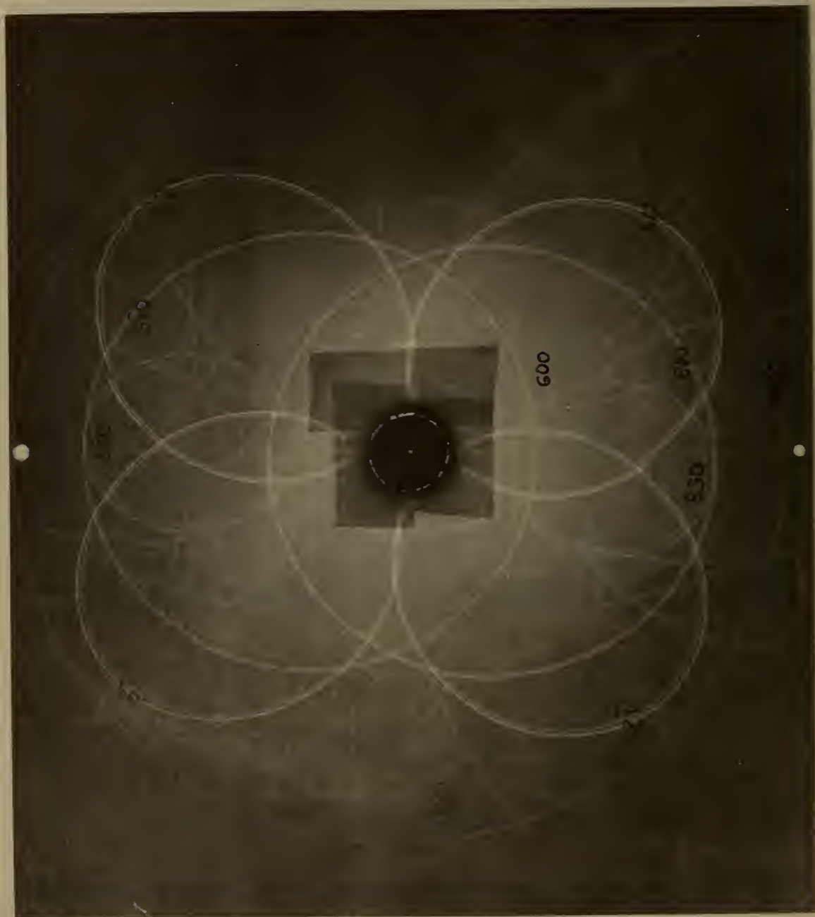
Figure 18. Back-reflection pseudo-Kossel line pattern from \text{TiO}_2 .
