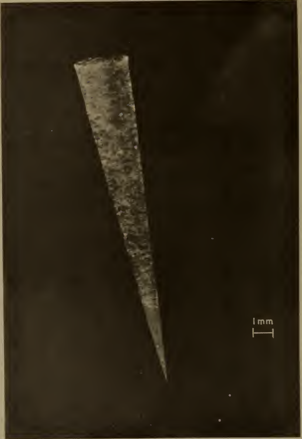
Figure 1. Lang Topograph of the best Al crystal so far produced.
