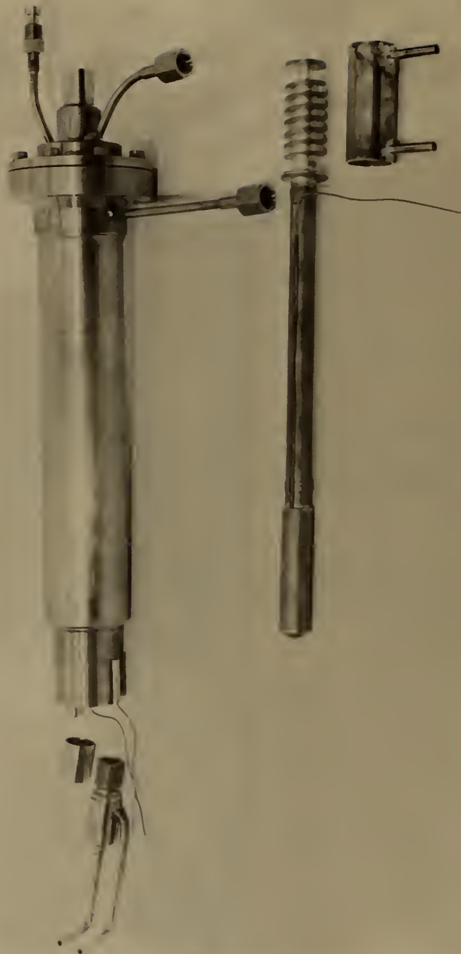
Figure 23. Assembled cell for use at 1000°C in phase purification.
