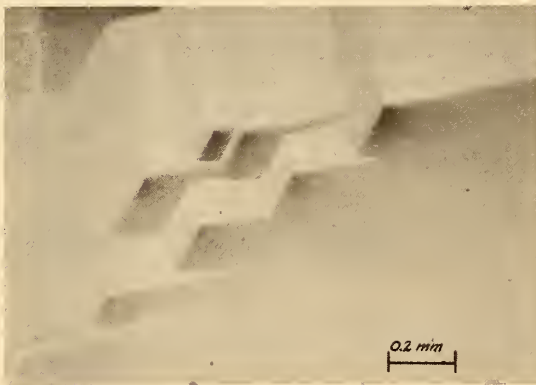
Fig. 8. Etch-pits in ADP [101]. Etchant: Same as for Figure 7.
