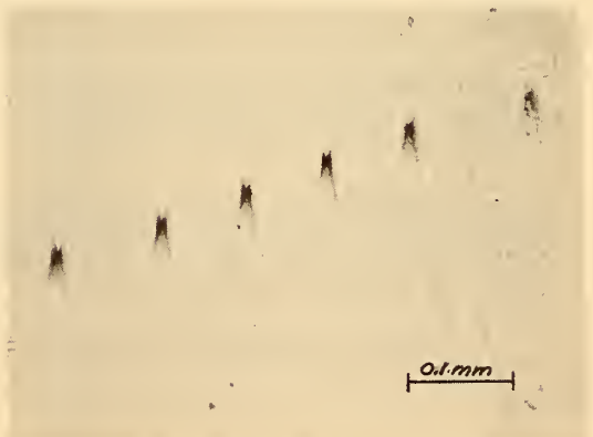
Fig. 9. Etch-pits in ADP [100]. Etchant: Saturated solution of potassium acid phthalate.
