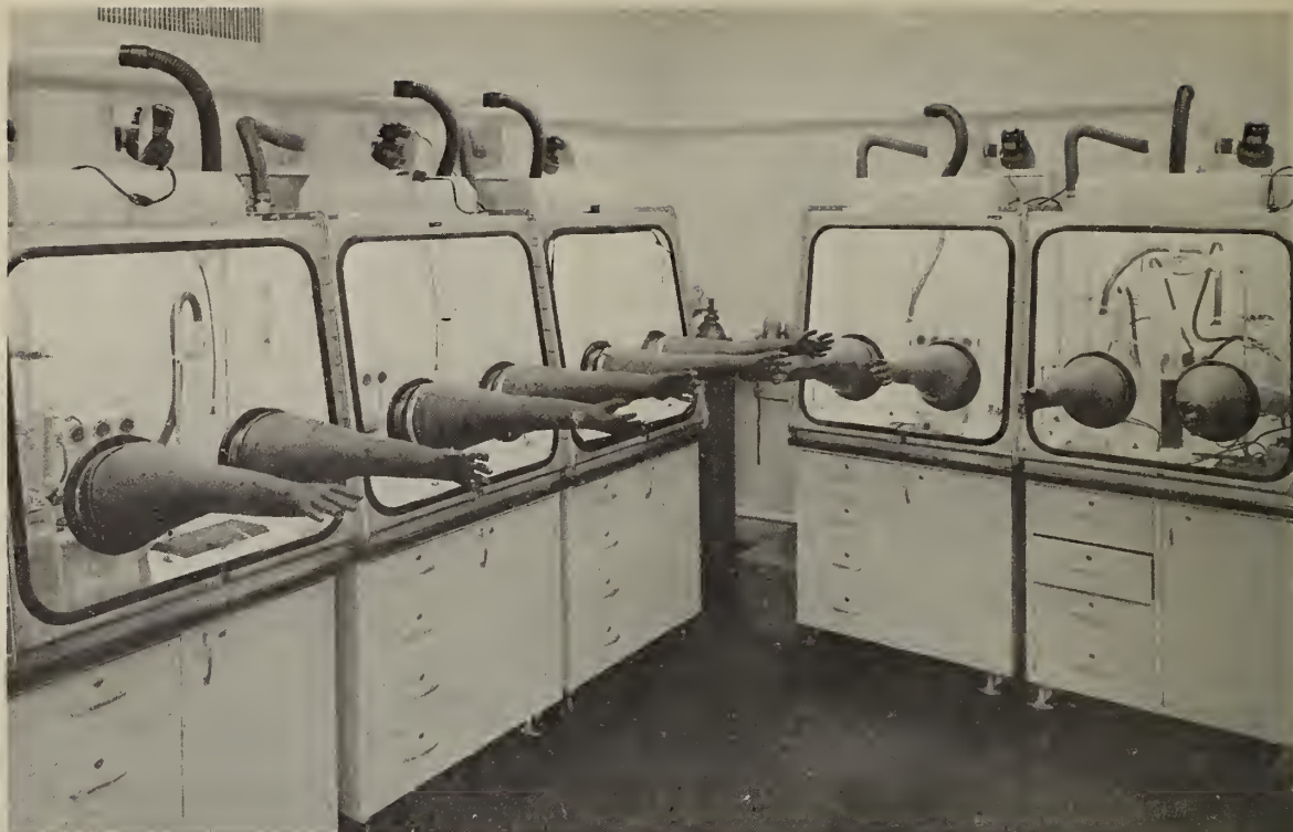
Figure 2. Glove box facility in clean room.
