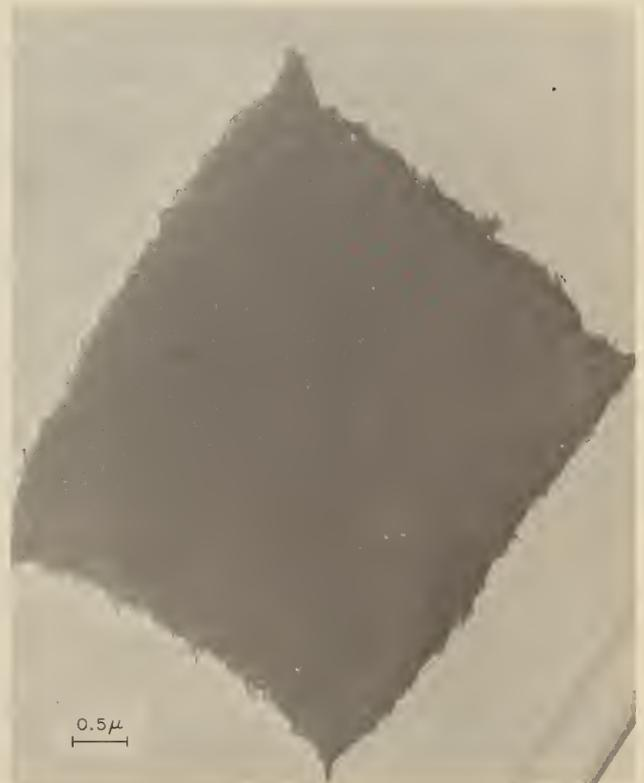
Fig.9 Transmission electron micrograph of a polypropylene aggregate exhibiting its pseudopolyhedral habit and fringe-like peripheral morphology.
