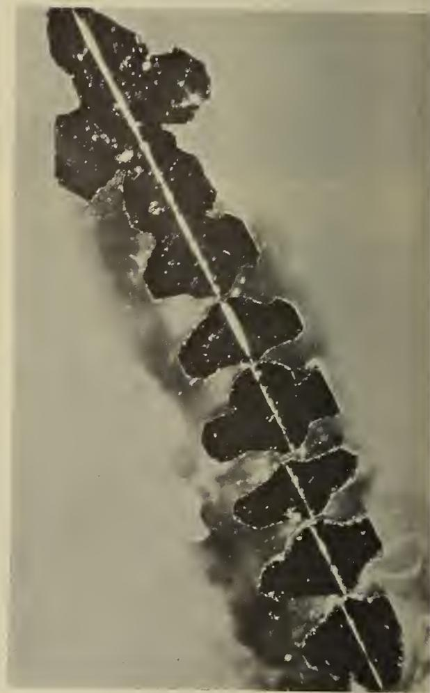
Fig. 17 Section of copper dendrite showing twin boundary
