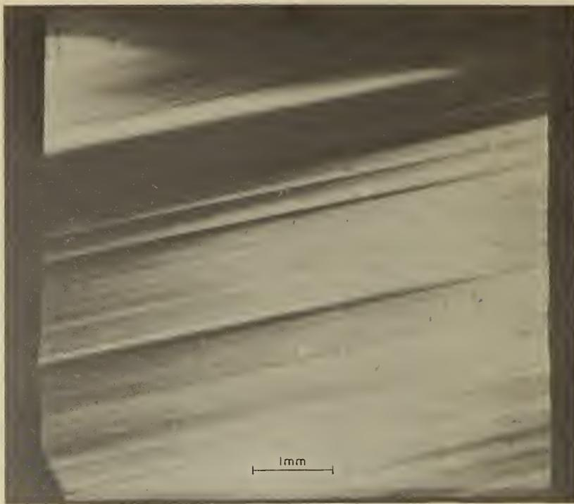
Fig. 20 Double-crystal diffraction topograph from a pair of natural quartz specimens. The samples were cut parallel to a set of  $\{11\bar{2}0\}$  planes, ground, polished, and etched for 20 minutes in 35% HF
