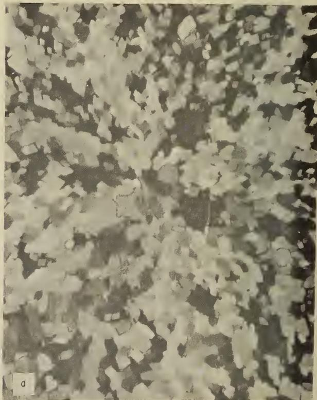
Fig. 7 Spherulites of 1,2-diphenylethane, showing crystallization phenomenon which occurs at room temperature. (a) Spherulite formed in alcohol bath, cooled to  $-75^{\circ}\text{C}$ ; (b) after 1/2 min atm. T (c) after 1 min atm. T (d) after 6 min atm. T
