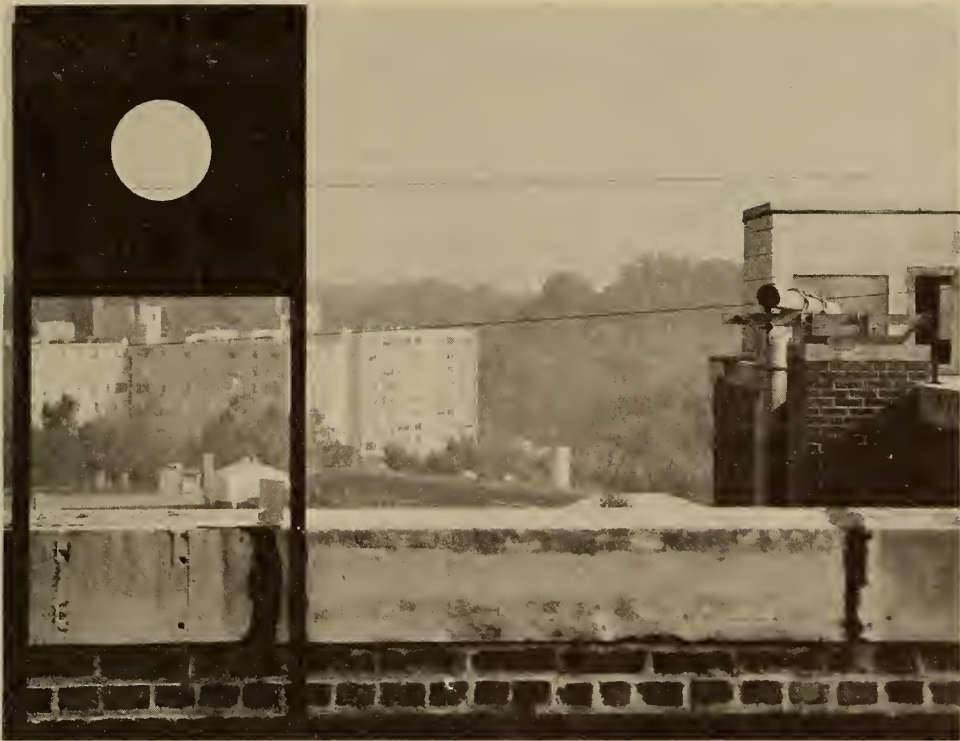
Figure 4A THE BAFFLING TUBE OF THE 279-METER RANGE- Seen are the baffling tube and one of the two other baffles.
