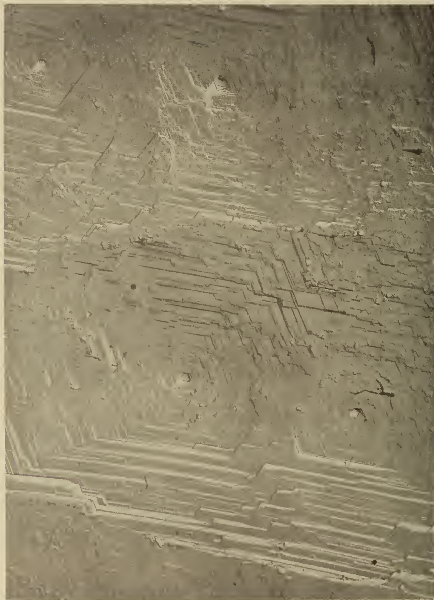
Figure 6. Electron micrograph of a shadowed carbon replica from a thermally evaporated {0001} zinc surface, illustrating the step structure at evaporation pits. Magnification = 4400.
