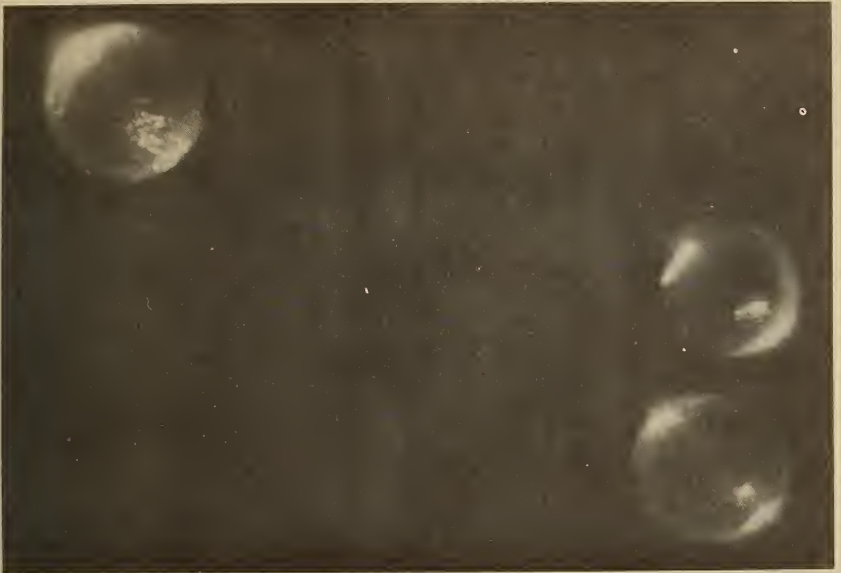
Figure 1. Individual polypropylene spherulites grown from a 10% solution of the polymer in xylene. The spherulites are shown as seen after evaporation of the solvent. (Unpolarized oblique incident illumination x 400).
