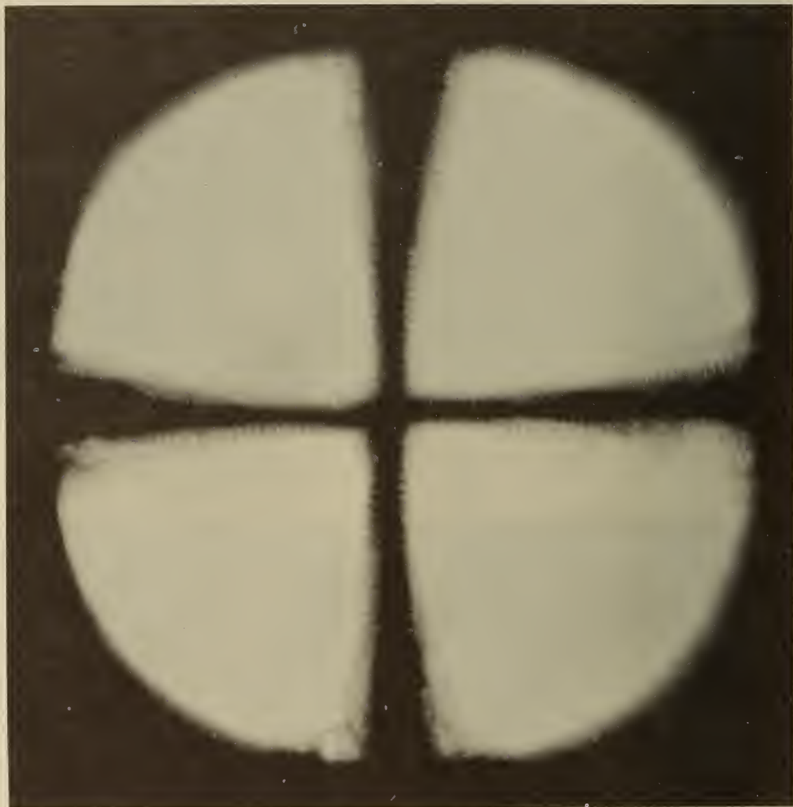
Figure 4. Spherulite of polyhexamethylene adipamide (66 nylon) grown from a 10% solution of the polymer in glycerol. The spherulite is in suspension in the solvent. (Crossed Nicols x 1500).
