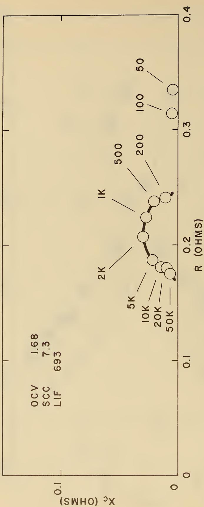
FIG. 31 RESISTANCE-REACTANCE CURVE OF GENERAL-PURPOSE D-SIZE CELLS OF BRAND 3 BEFORE DISCHARGE
