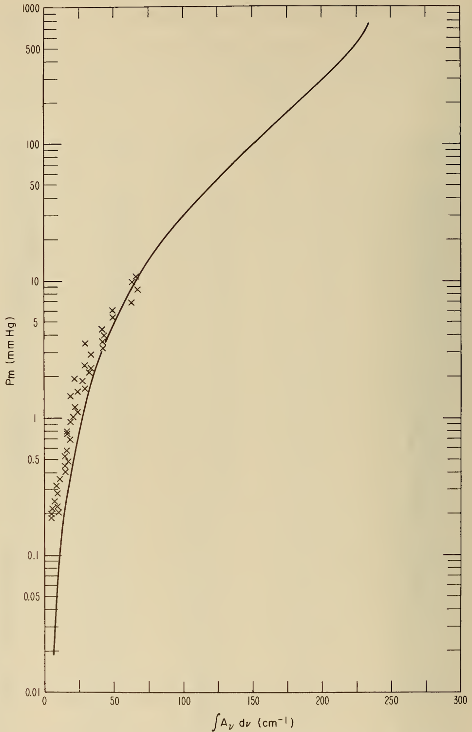
Figure 2. Atmospheric absorption of the 2.7\mu band of CO 2 is shown as a function of pressure. The data obtained from the balloon flight of Murcray et. al, are represented by x. An isothermal atmosphere is assumed.
