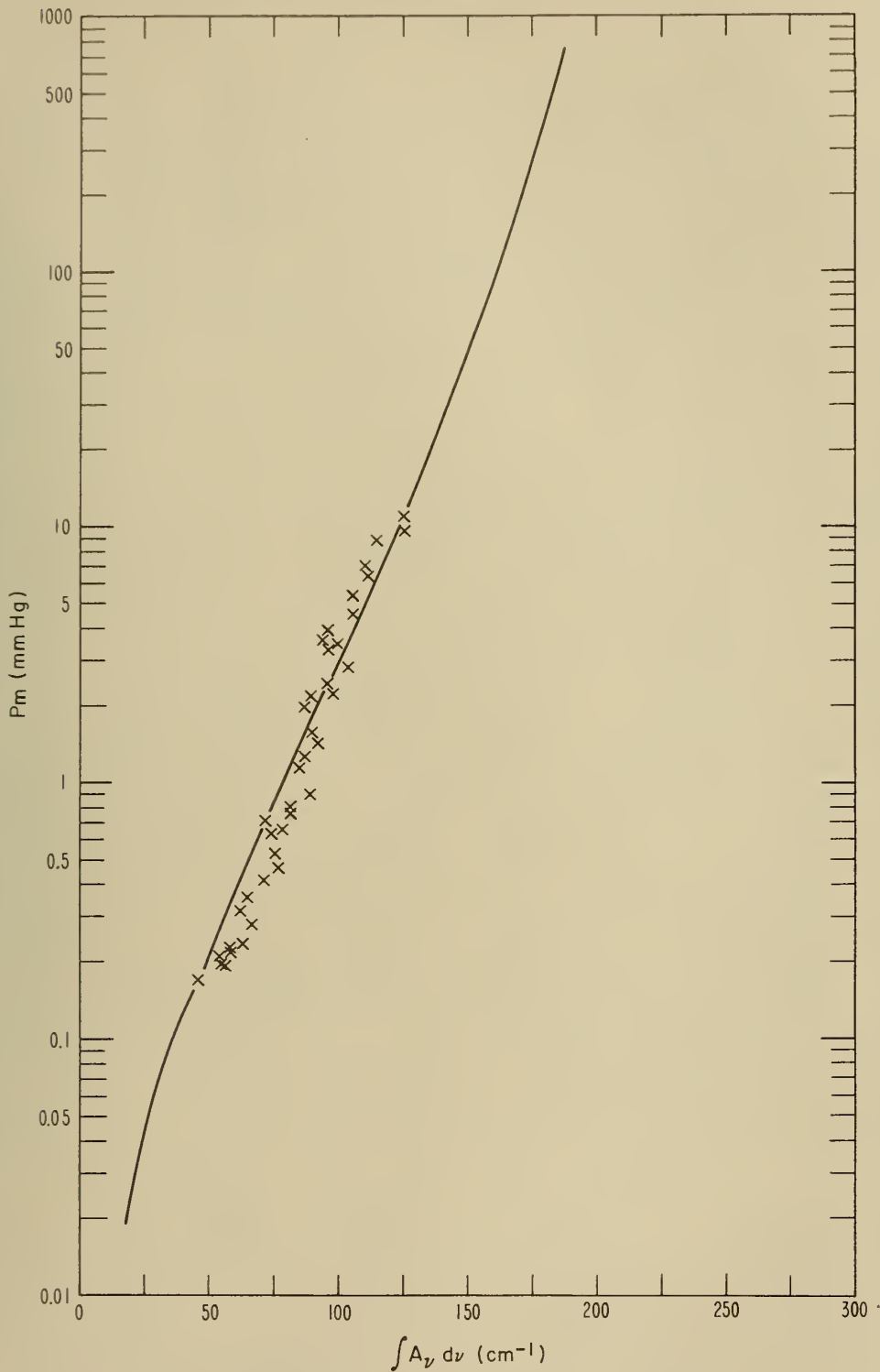
Figure 3. Atmospheric absorption of the 4.3\mu band of CO 2 is shown as a function of pressure. The data obtained from the balloon flight of Murcray et. al. are represented by x. An isothermal atmosphere is assumed.
