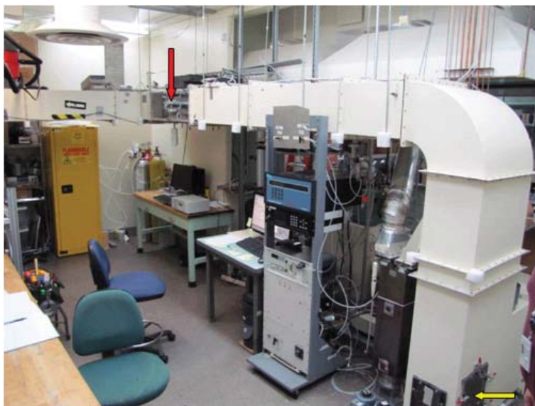
FIGURE3: PHOTOGRAPH OF THE FIRE EMULATOR/DETECTOR EVALUATOR Note: The red arrow denotes the test section and the yellow arrow denotes the smoke source.
