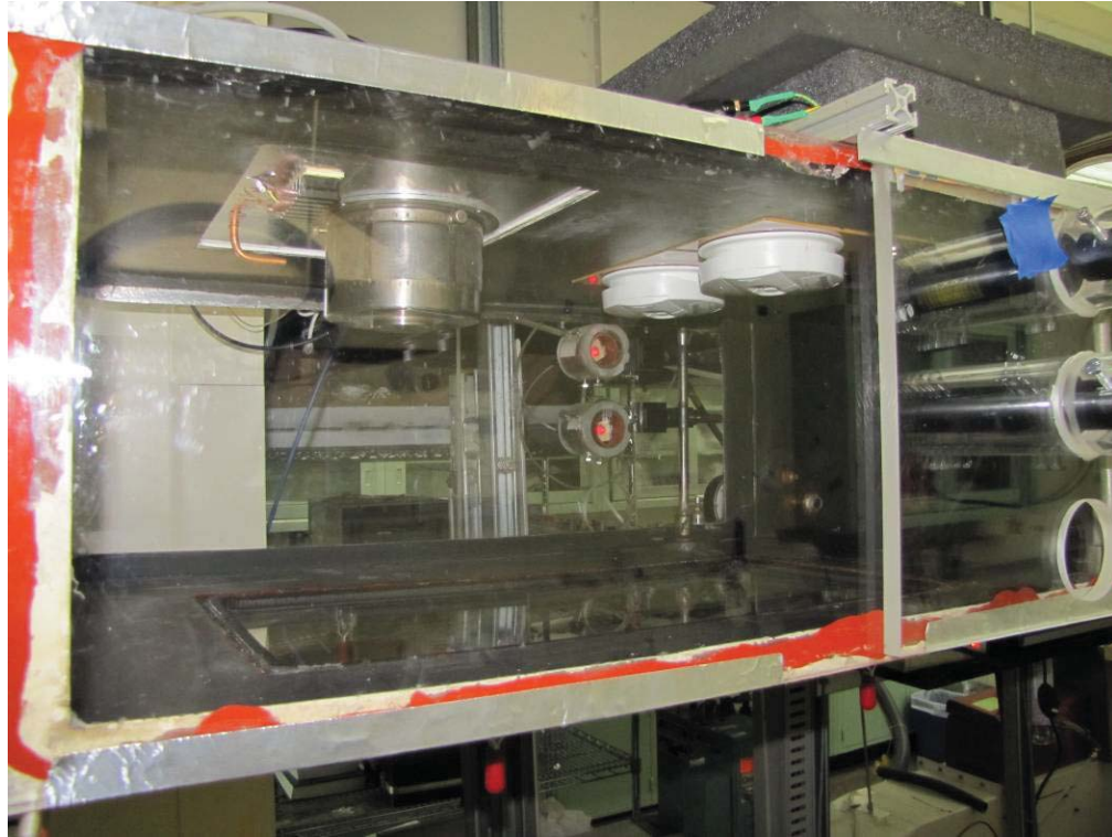
FIGURE 4: CLOSE-UP OF THE TEST SECTION, SHOWING TWO CEILING-MOUNTED SMOKE ALARMS AND TWO LASERS FOR SMOKE OBSCURATION MEASUREMENT
