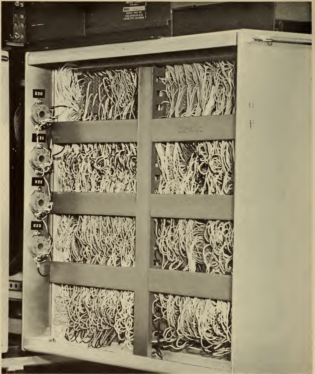
FIGURE 24. WIRING SIDE OF A TYPICAL DRAWER CHASSIS
