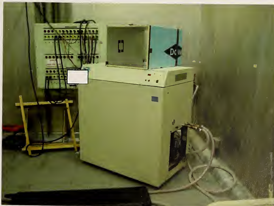
Figure B12: Portable water chiller connected to house water and used to control water temperature fed to the water-cooled condensing unit
