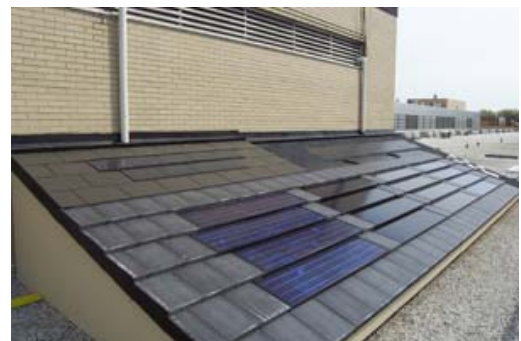
NIST's outdoor residential photovoltaic test facility is used to collect performance data for model improvement and validation. (Photo: NIST)
