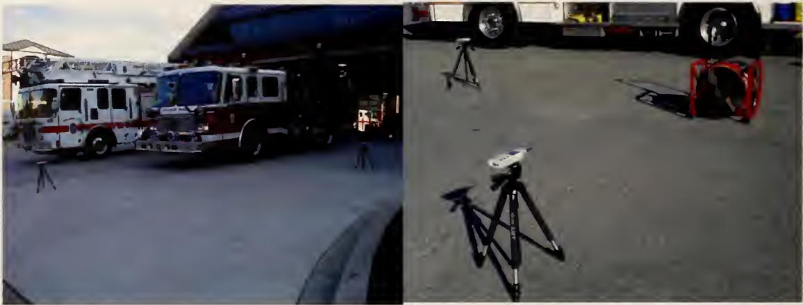
Figure 16. Photographs showing background sound level measurement tests.
