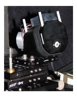
Fig. 6. Picture of the sphere-InGaAs detector.
