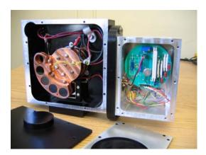
**Figure 1.** Picture of the prototype singleelement-Si based colorimeter
