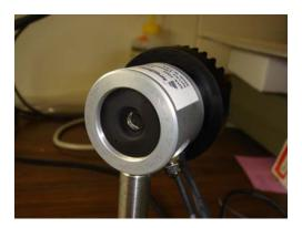
Fig. 1. A temperature-controlled pyroelectric transfer-standard radiometer head.
