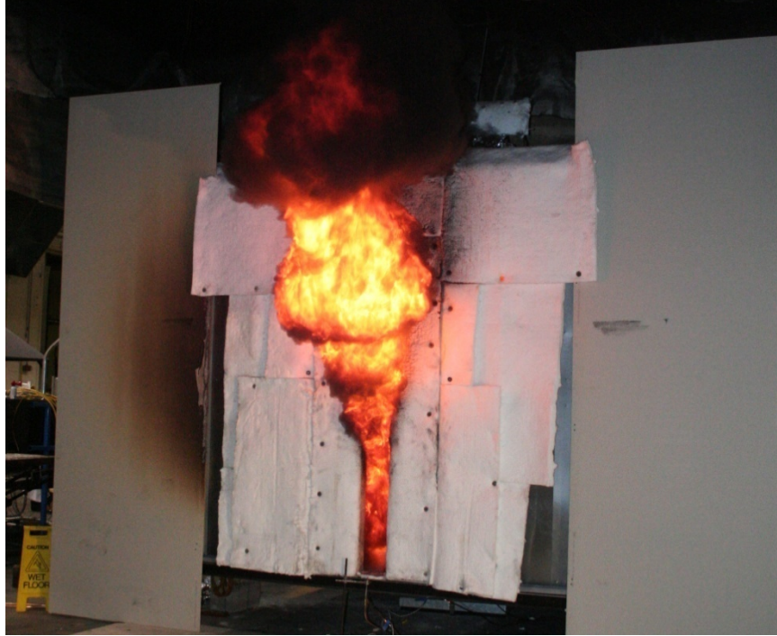
Figure 3.7: Fire leaving the door of the ISO 9705 room during test ISOHeptD12. It was not possible to view the inside of the room during this test.
