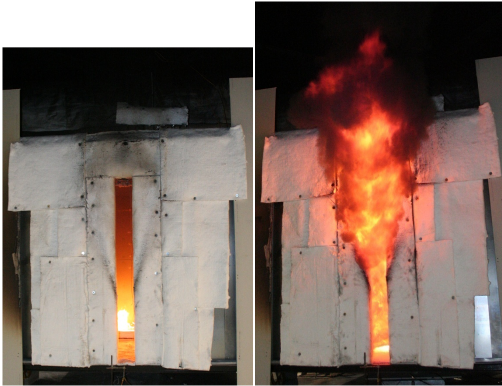
Figure 5.1: Example normalized scaling quantities with Q_d^* = 0.17 , \phi = 0.1 , and H/D^* = 12.23 , on the left (ISONylon10) and a Q_d^* = 12.74 , \phi = 7.53 , and H/D^* = 2.17 , on the right (ISOPropD14).
