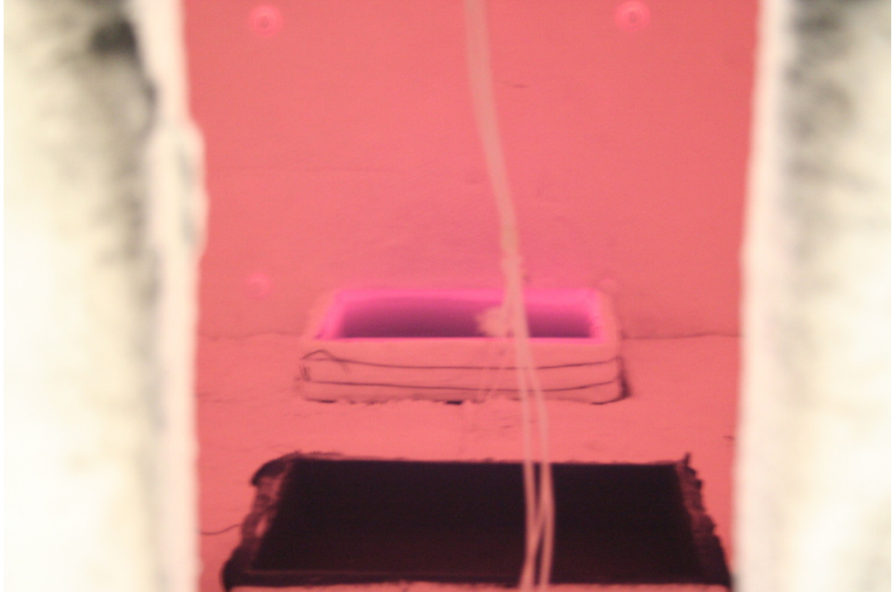
Figure 3.24: Photograph of the center (front) and rear burners immediately after fire test ISOPropD14.
