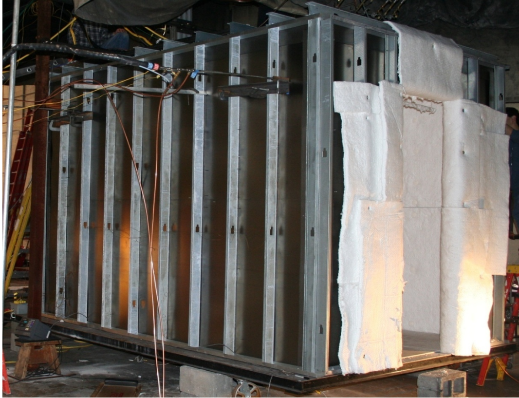
Figure 2.2 Photograph of the actual ISO 9705 room used for experiments. The structural construction of sheet steel on steel studs can be seen along with the internal surface covering of ceramic fiber blanket.
