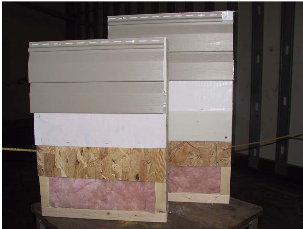
Figure 5. Photograph showing structural differences between unrestricted (left) and fire resistant (right) construction.
