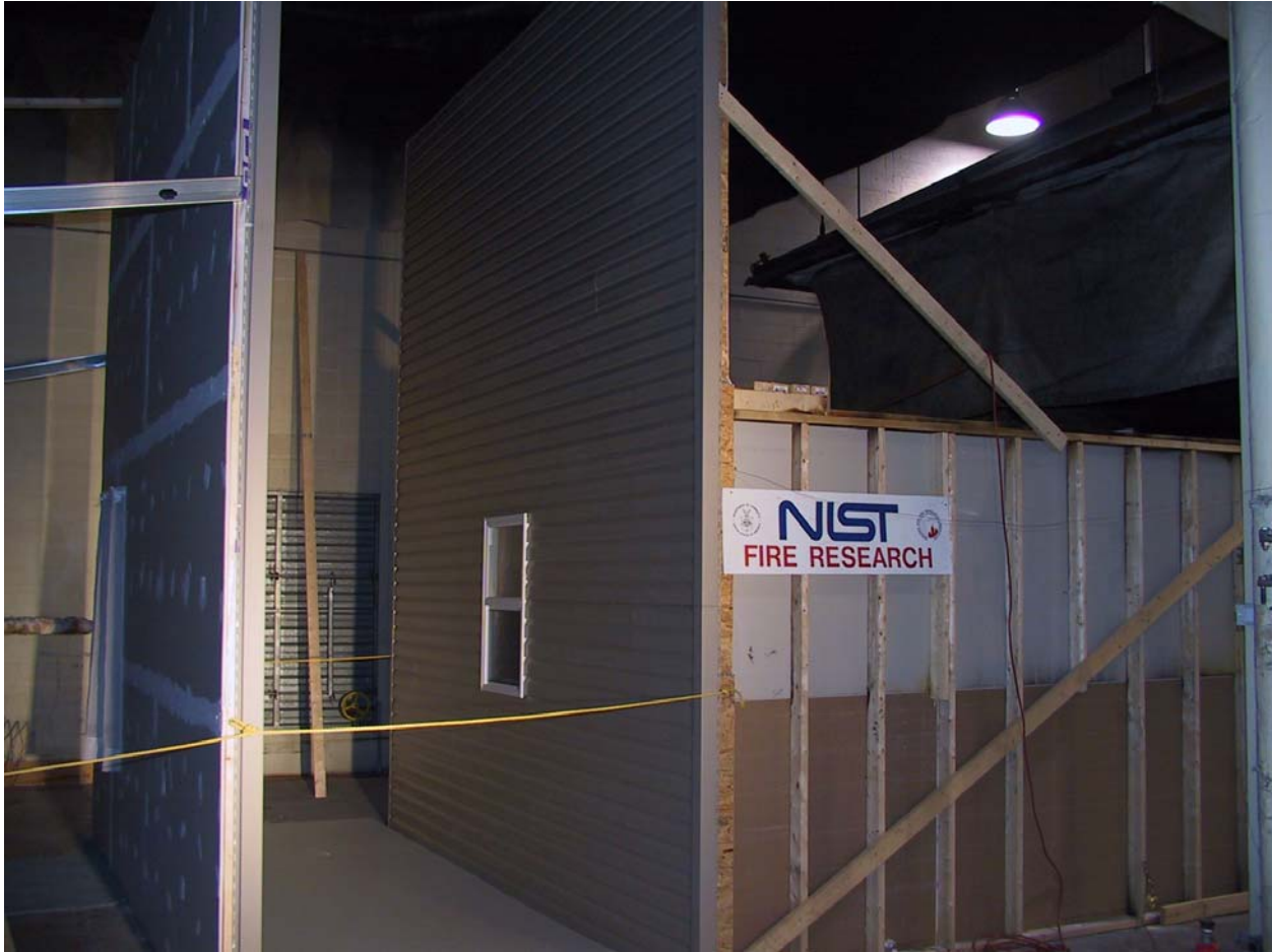
Figure 1. Photograph of the side of the structure of origin facing the adjacent target wall.
