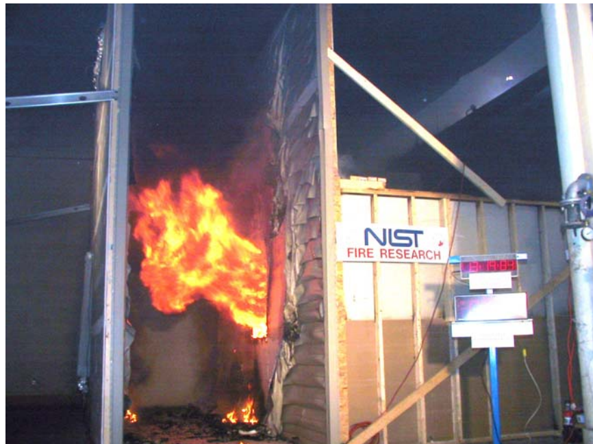
Figure 16. Fire Resistant Construction Experiment: 9 min after Window Failure – Target Wall OSB Not Ignited
