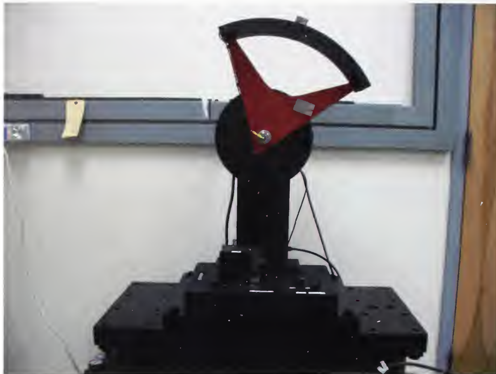
Figure 5 - General view of the NIST small-scale table-top instrumented impact tester.
