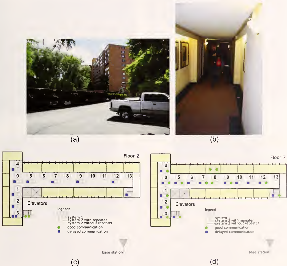
Figure 3.2: (a) 12-story apartment building Horizon West. (b) Inside on Floor 7. (c) Test positions on Floor 2. (d) Test positions on Floor 7. Blue squares indicate a delay in the reception of the alarm signal. Green circles indicate reception without significant delay.
