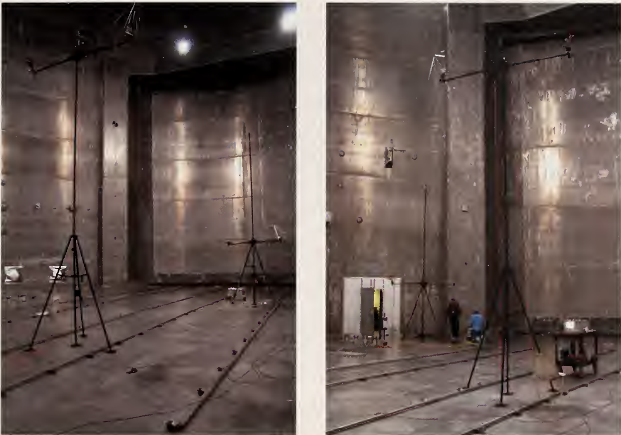
Figure 43. Two examples of the test configuration used to position the antennas during the empty chamber tests at the low- and mid-band frequencies.
