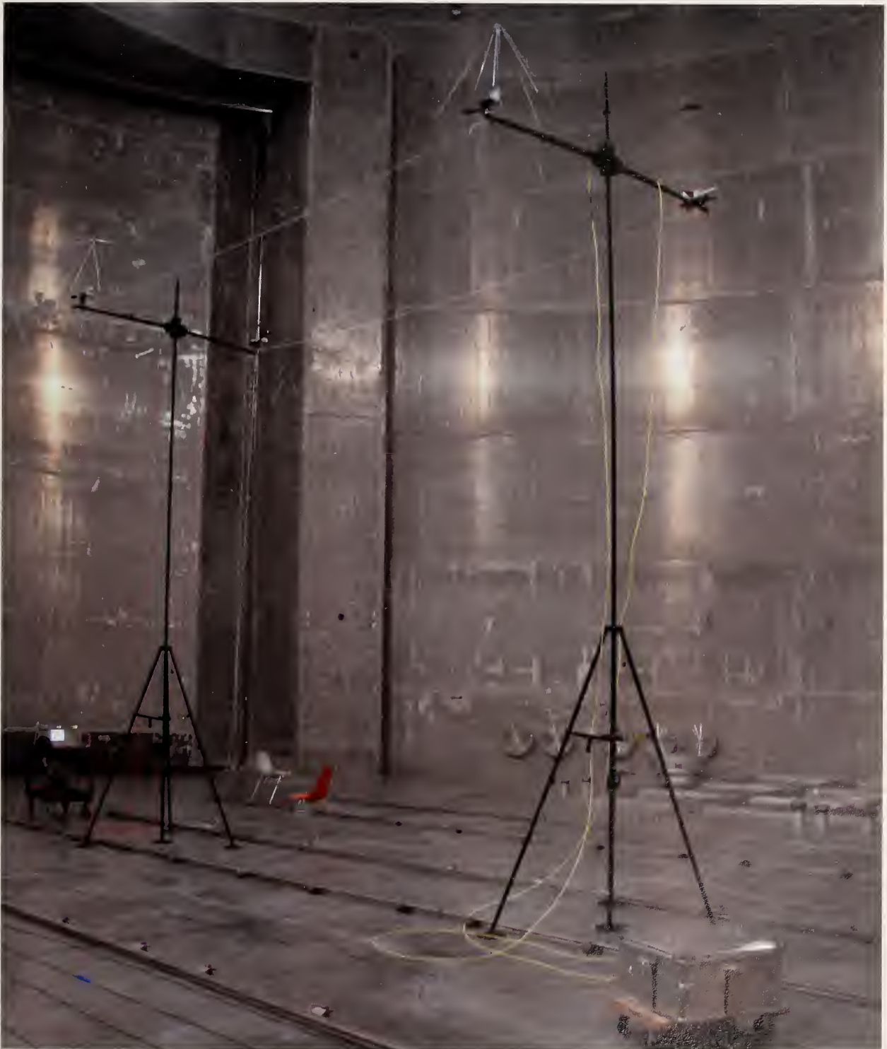
Figure 40. Initial attenuation measurements near the center of the chamber with antennas' polarization matched and aligned to bore sight.
