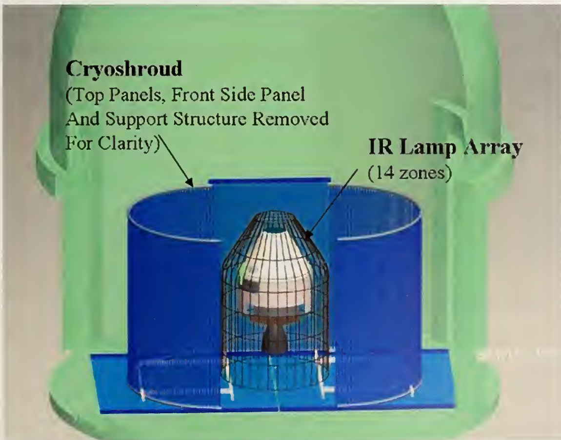
Figure 21. Artist's rendering of the bottom portion of the space vehicle inside an infrared (IR) Lamp array and the cryoshroud. (Drawing courtesy of NASA)
