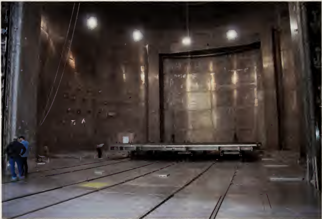
Figure 46. The cryo-floor assembly is positioned in the center of the SPF aluminum chamber prior to closing the large access door.
