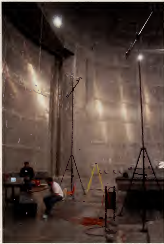
Figure 52. Photographs of typical transmit and receive antenna positions while testing at positions on the chamber floor.
