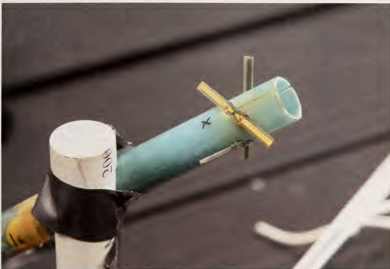
Figure 37. Close-up of one of the 5 cm dipole probes. The diode detector is under the small black dot at the center gap of the dipole. The black material is opaque epoxy covering the diode to prevent photo effects in the diode response.
