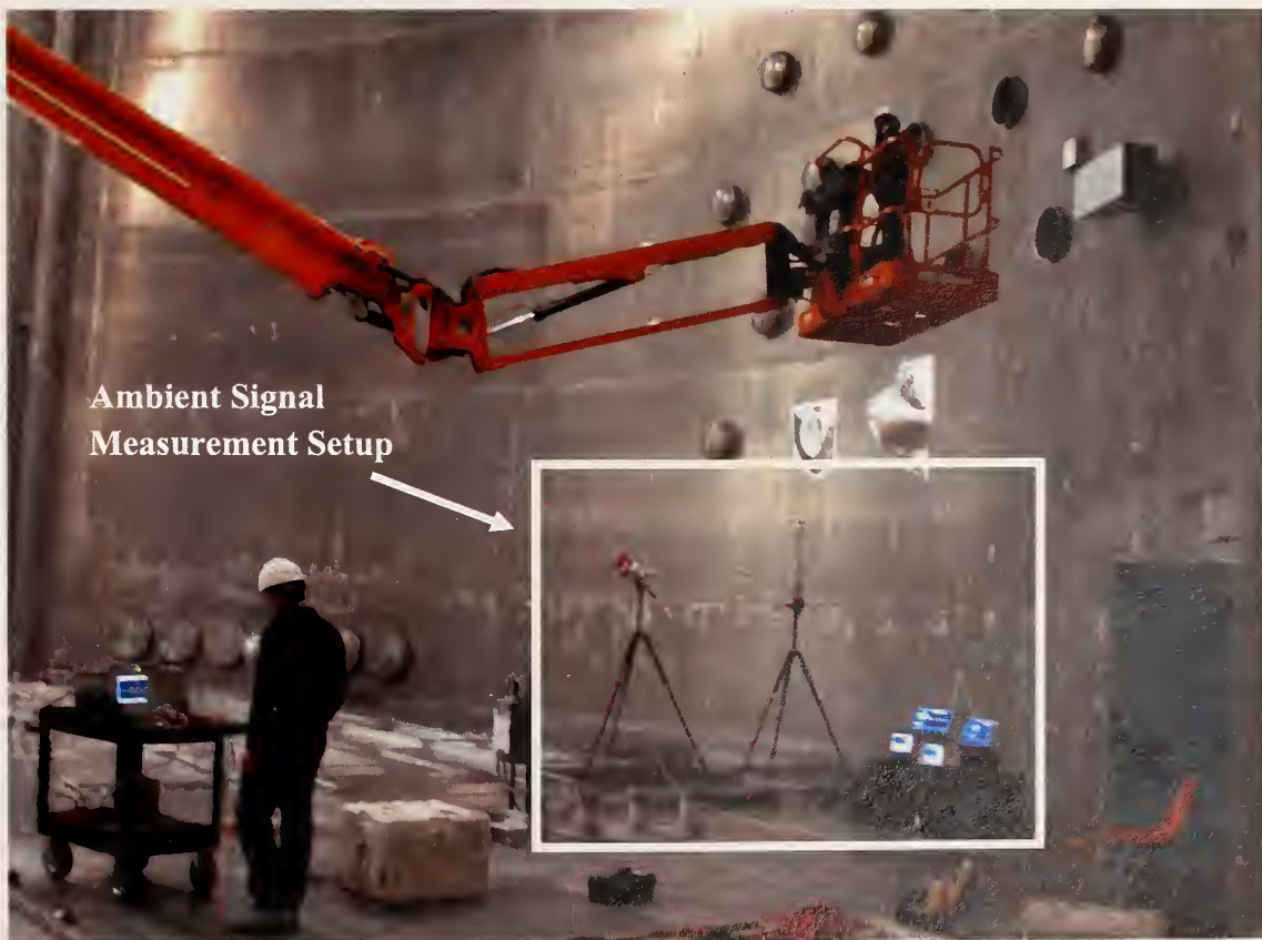
Figure 94. Ambient signal measurement setup of two spectrum analyzers. One with a dual ridged horn (red in color) and the other with a discone antenna. Each connected to a laptop for recording data.
