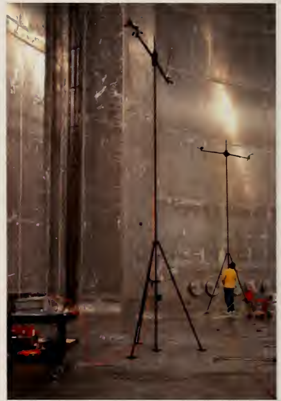
Figure 52. Photographs of typical transmit and receive antenna positions while testing at positions on the chamber floor.
