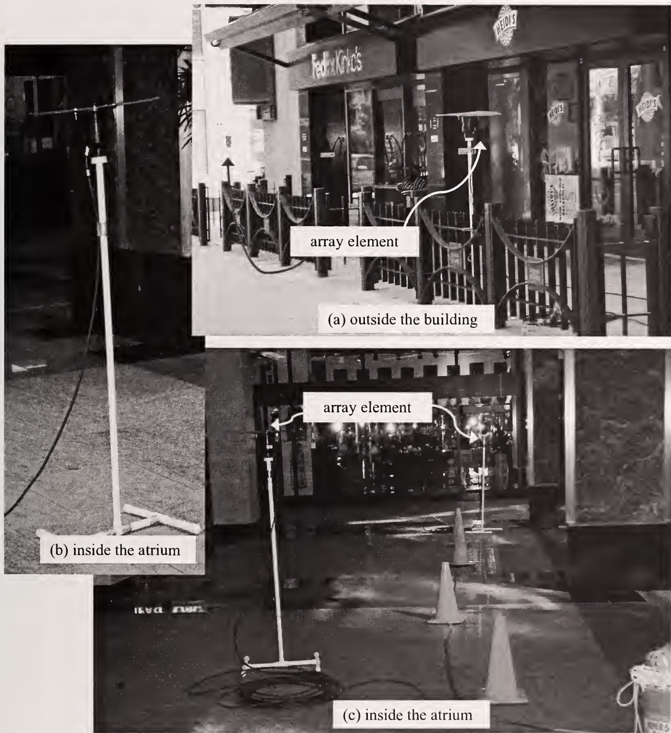
Figure 4. Some of the 2.4 GHz antennas used in the 2.4 GHz experiments at the Denver location, both inside and outside of the atrium area.
