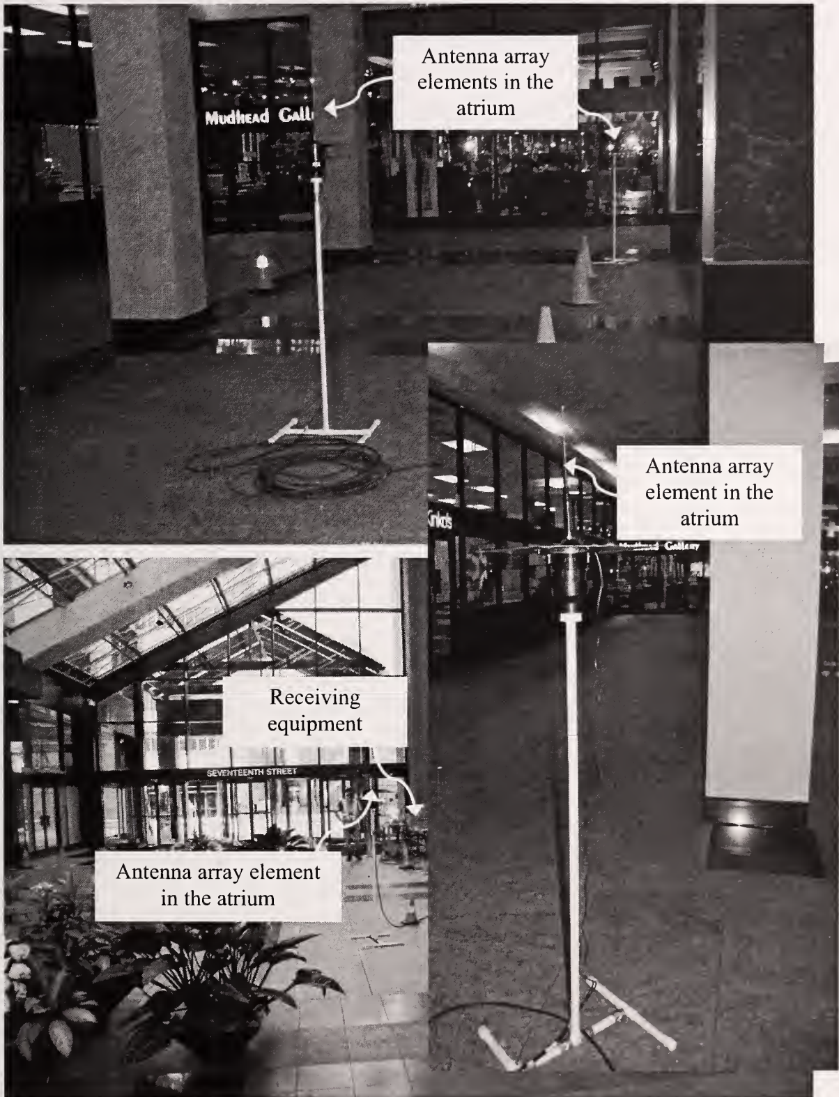
Figure 8. Some of the antenna array elements used in the 750 MHz measurements carried out in Denver.
