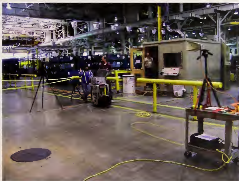
Figure 5-5: Photograph looking the other way in the same corridor of the stamping plant. The high-frequency directional antennas are shown. The photograph shows the VNA and the optical fiber linking the transmitting and receiving antennas.
