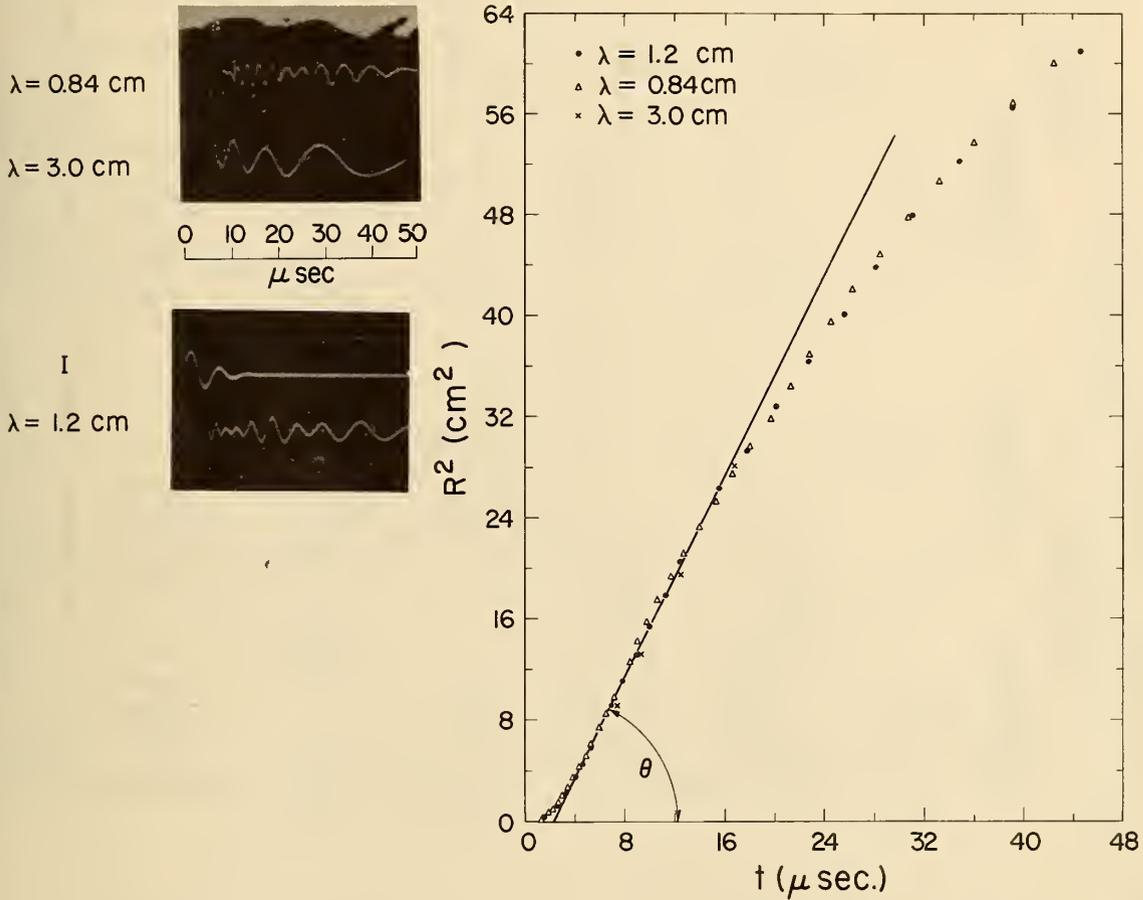
Figure 1. Oscilloscope traces of microwave Doppler measurements of the expanding cylindrical shock front from a wire explosion, are shown on the left. A plot of the square of the radius of the ionization front with time is on the right. The straight line portion of the plotted points represents agreement with the theory. This explosion was made in air at a pressure of 30 cm Hg. The energy released into the 4 cm long, 18 mil copper wire was 500 joules per centimeter of wire length.
