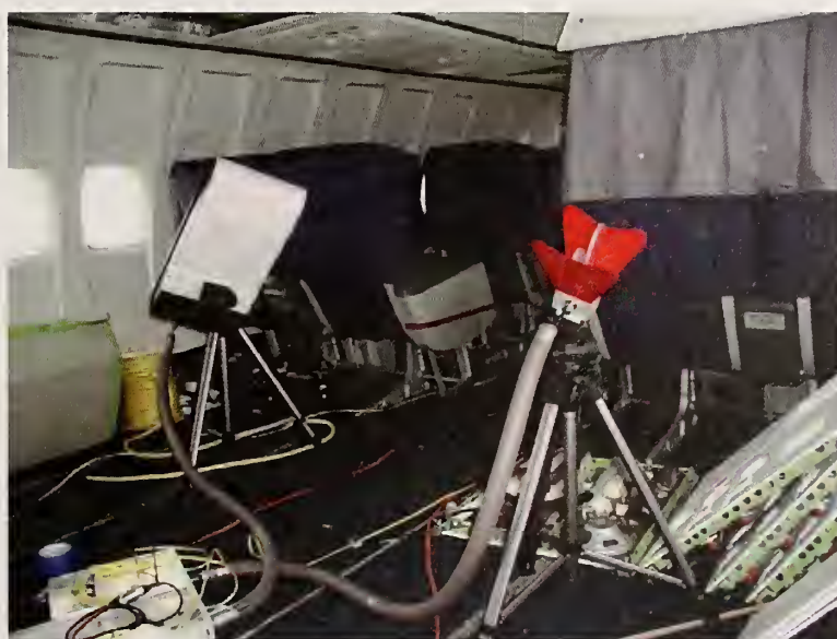
Figure 64. Placement of receiving DRG and TEM horn antennas in the mid-passenger cabin for position 2.
