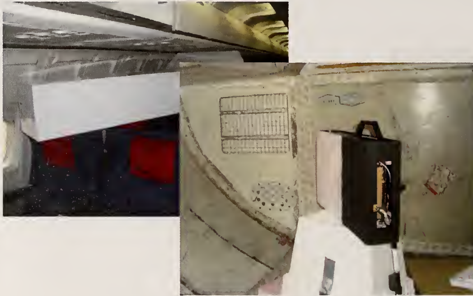
Figure 183. Main cabin to cargo bay TEM horn antenna setup 5.
