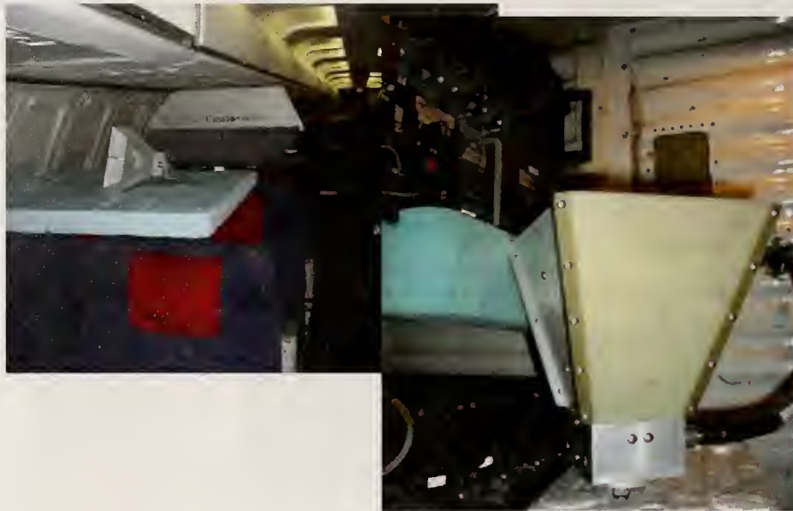
Figure 202. Main cabin to avionics bay DRG horn antenna setup 4.
