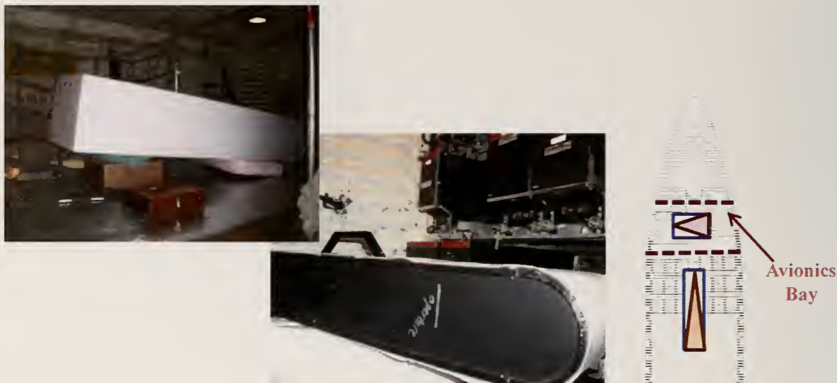
Figure 226. Cargo bay to avionics bay TEM horn antenna setup A.
