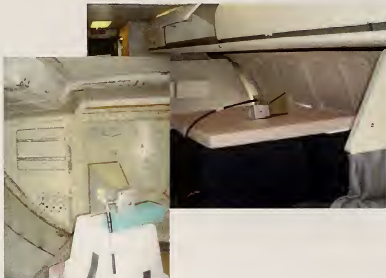
Figure 163. Main cabin to cargo bay DRG horn antenna setup 5.
