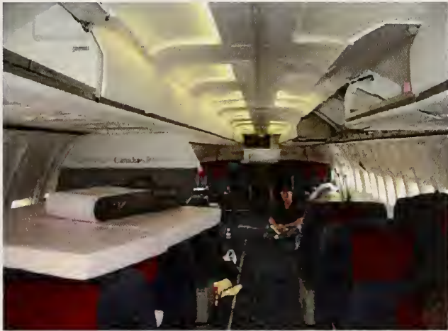
Figure 81. Main cabin to main cabin TEM horn antenna setup 1.
