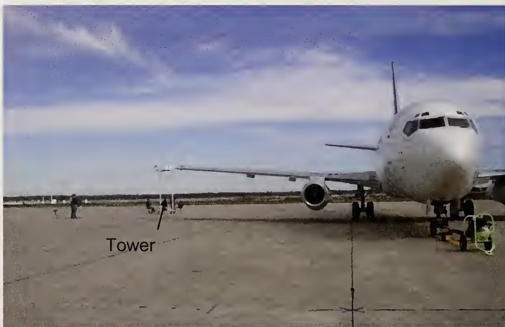
Figure 40. The transmitting antennas placed on top of a support tower and boresighted at the center of the aircraft.
