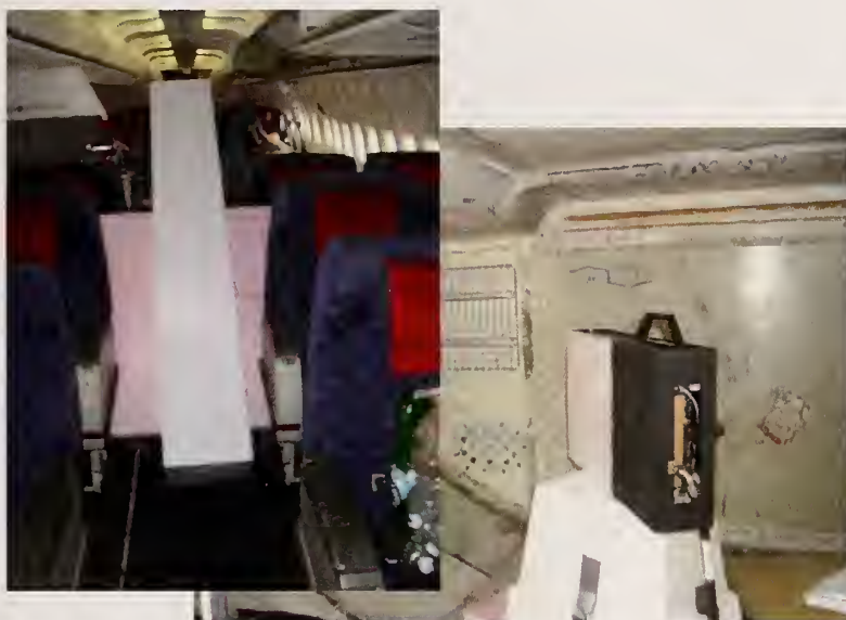
Figure 181. Main cabin to cargo bay TEM horn antenna setup 4.
