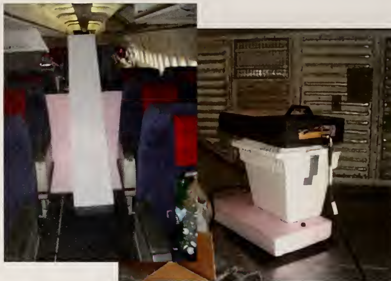
Figure 179. Main cabin to cargo bay TEM horn antenna setup 3.
