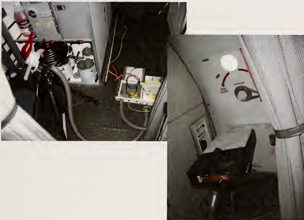
Figure 56. Placement of receiving DRG and TEM horn antennas in the front galley for position 3.
