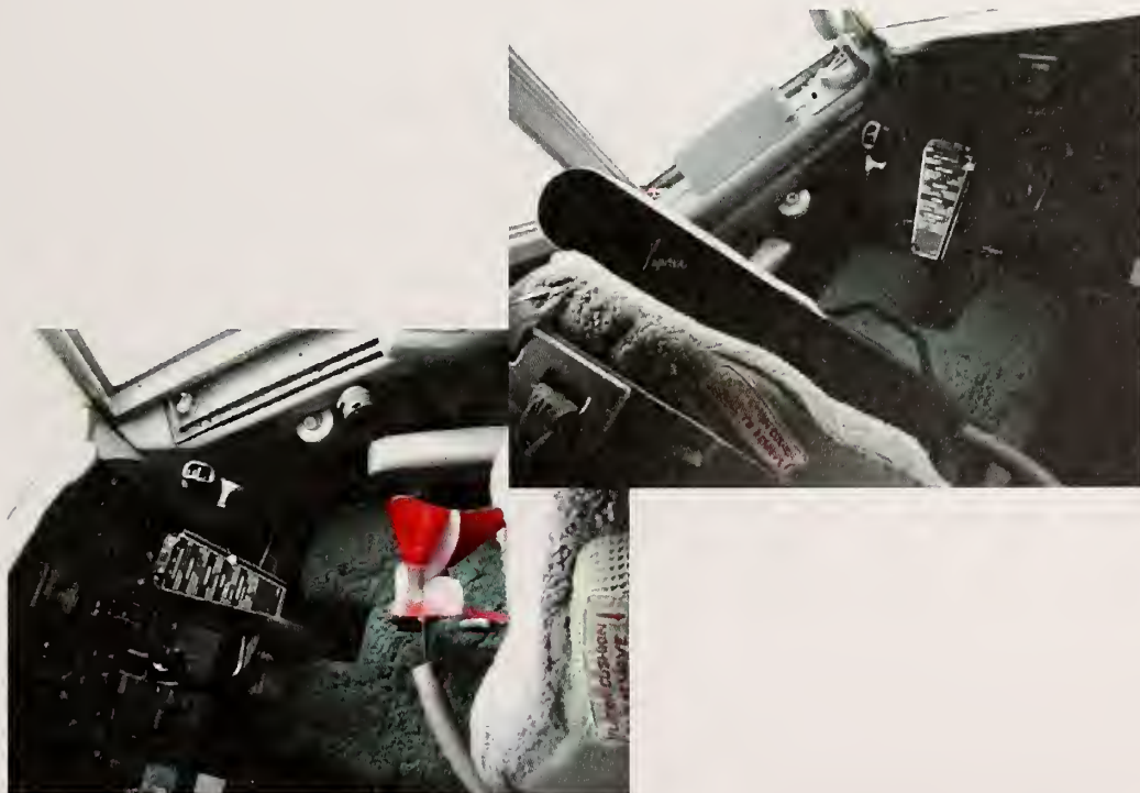
Figure 54. Placement of receiving DRG and TEM horn antennas in the flight deck for position 5.
