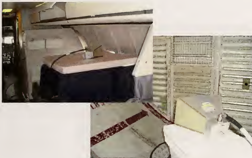
Figure 161. Main cabin to cargo bay DRG horn antenna setup 2.
