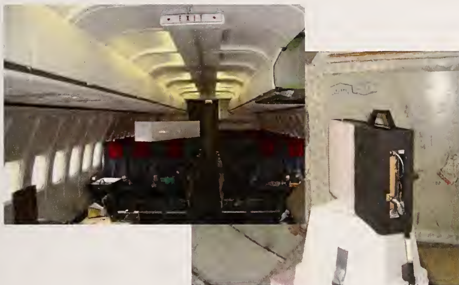
Figure 185. Main cabin to cargo bay TEM horn antenna setup 6.
