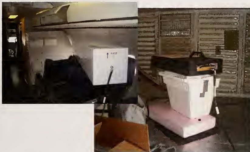
Figure 177. Main cabin to cargo bay TEM horn antenna setup 2.
