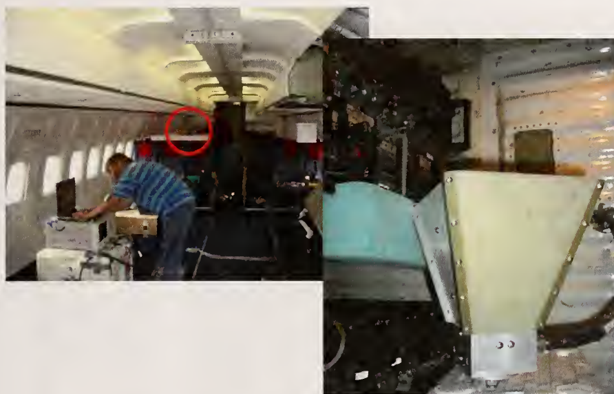
Figure 200. Main cabin to avionics bay DRG horn antenna setup 3.
