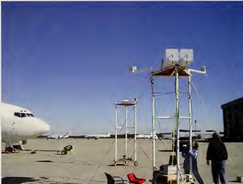
Figure 39. Reference measurement setup. The transmitting tower is configured for all measurements, and the receiving tower is configured for reference measurements only.
