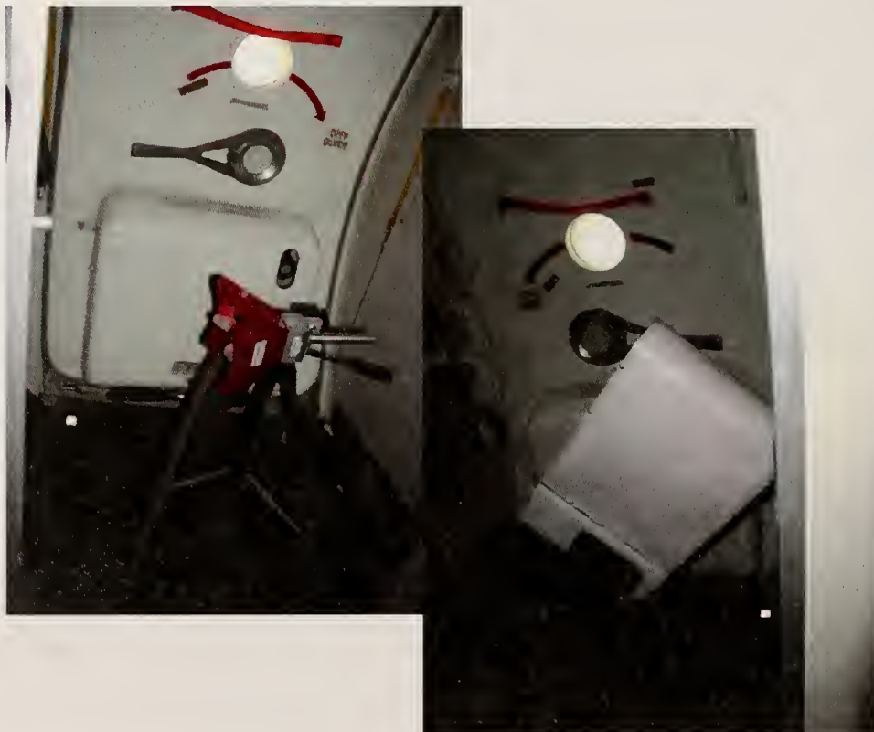
Figure 60. Placement of receiving DRG and TEM horn antennas in the rear galley for position 7.
