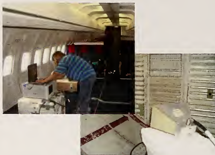
Figure 159. Main cabin to cargo bay DRG horn antenna setup 1.
