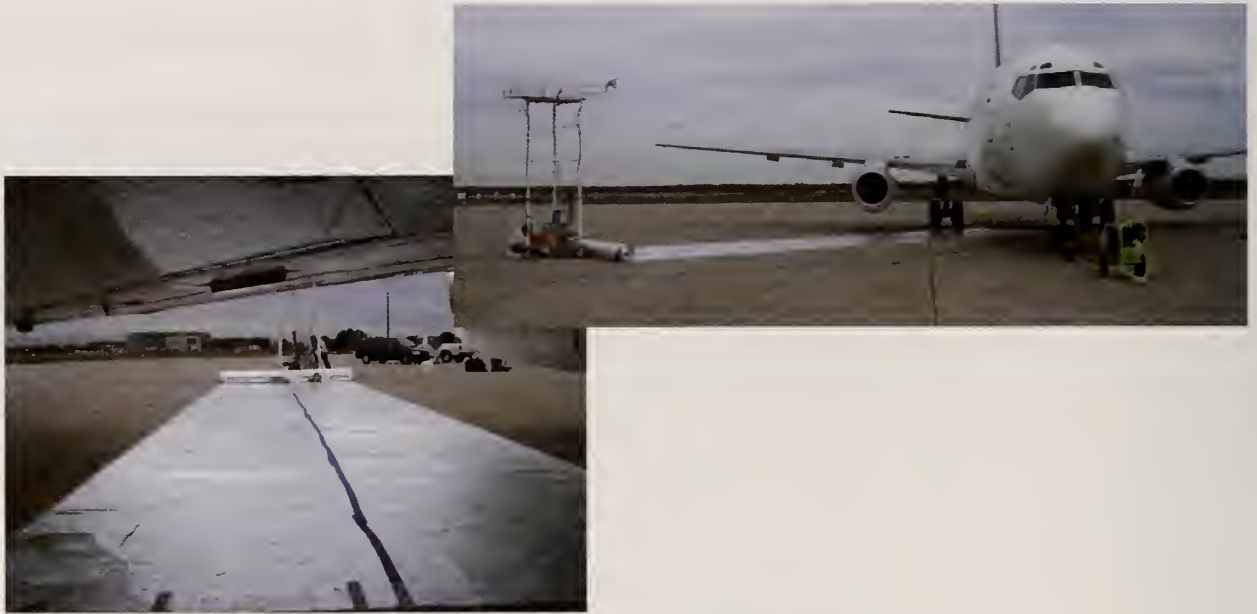
Figure 28. Photographs showing Rfoil laid out beneath aircraft for the various ground condition experiments.
