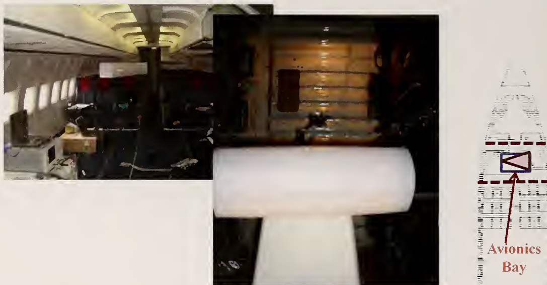
Figure 211. Main cabin to avionics bay TEM horn antenna setup 1.
