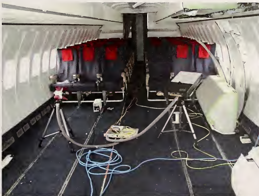
Figure 69. Placement of receiving DRG and TEM horn antennas in the mid-passenger cabin for single-position quadrant measurements looking toward rear of aircraft.
