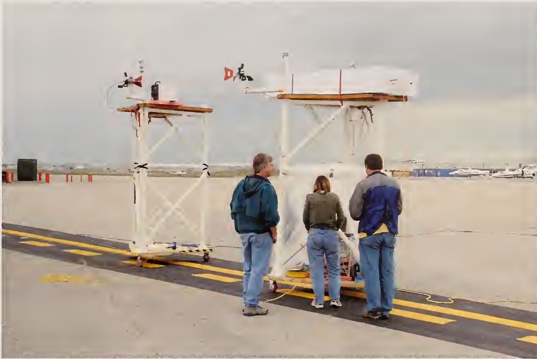
Figure 6. Reference measurement setup. The transmitting tower is configured and the receiving antennas will be mounted on top of the second tower.
