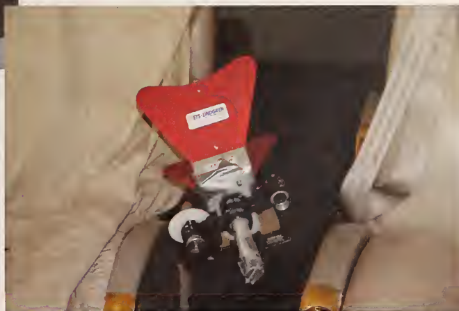
Figure 110. Layout for DRG configuration 4 measurements. One antenna points out of the left window in the flight deck. The second antenna points into the middle lefthand seat.
