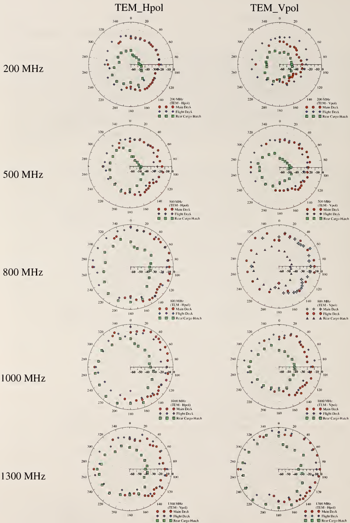
Figure 124. Graphs for TEM horn antenna in both vertical and horizontal polarizations for various frequencies in each compartment. Red circles (●) are for the main cabin, blue diamonds (◆) are for the flight deck, and green squares (■) are for the rear cargo hatch.
