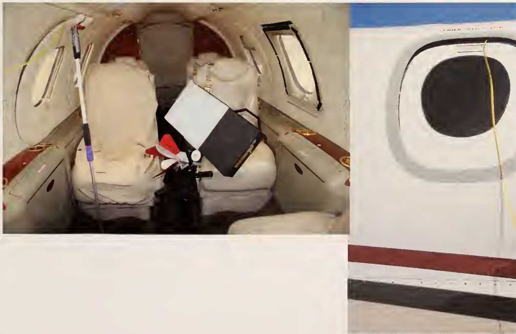
Figure 19. Receiving antenna placement in main passenger cabin.
