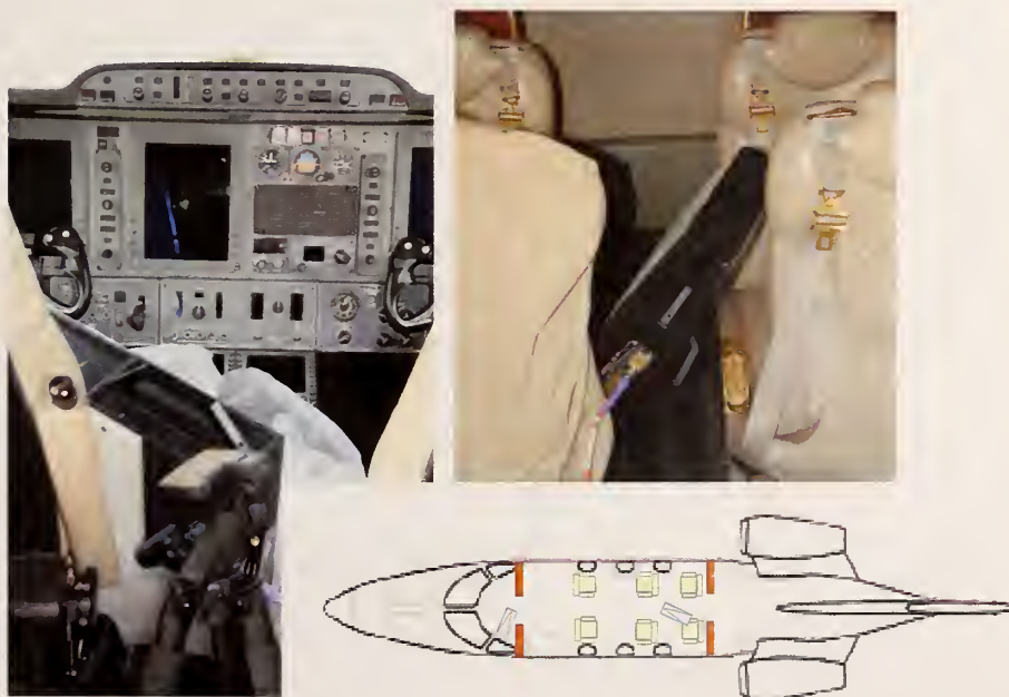
Figure 114. Layout for TEM configuration 3 measurements. One antenna points out the righthand window of the flight deck. The second antenna points toward the right rear seat.
