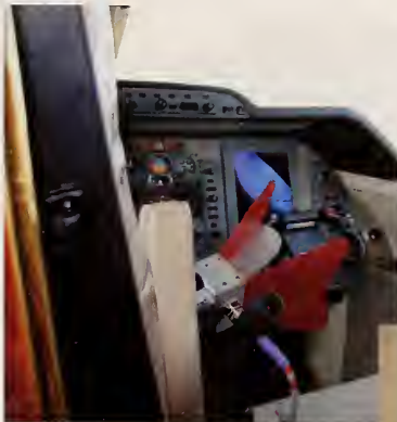
Figure 109. Layout for DRG configuration 3 measurements. One antenna points out of the left window in the flight deck. The second antenna points into the last lefthand seat.
