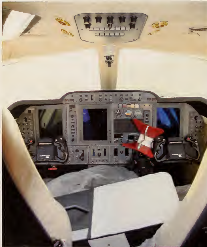
Figure 51. The receiving DRG and TEM antennas placed between the pilot's and co-pilot's seat.
