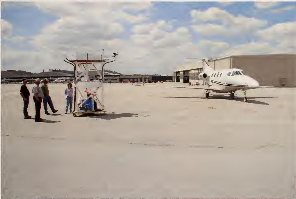
Figure 7. The transmitting antennas placed on top of a support tower and boresighted at the center of the aircraft.
