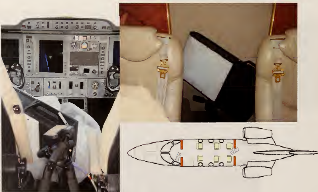
Figure 111. Layout for DRG configuration 5 measurements. One antenna points toward the first, lefthand window in the passenger cabin. The second antenna points into the middle lefthand seat.
