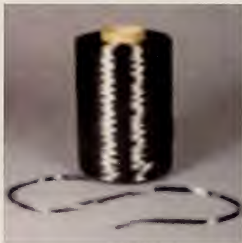
Figure 136. Spool of carbon fiber strand [12].
