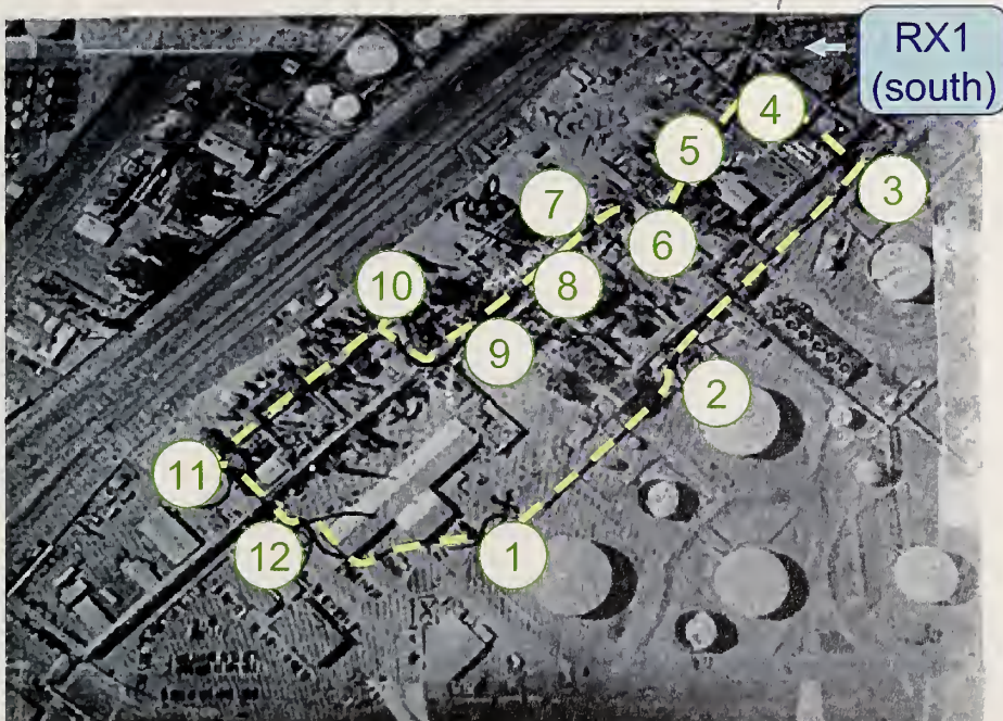
Figure 5.2-1: Path taken through the complex in measurements of narrowband received power. Portable transmitters were carried along the path shown by the green dashed line, and the received signals were measured at the location marked “RX1.” At point 9, NIST staff climbed approximately 30 m up a tower.
