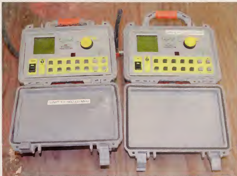
Figure 2. Transmitters used for the higher frequency bands.
