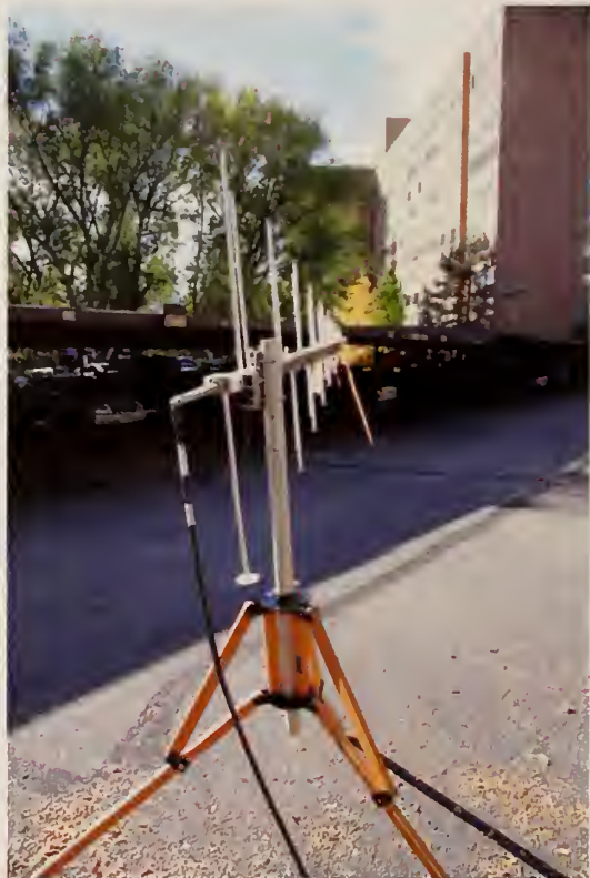
Figure 36. Receiver setups for Horizon West apartment building in Boulder, CO.
