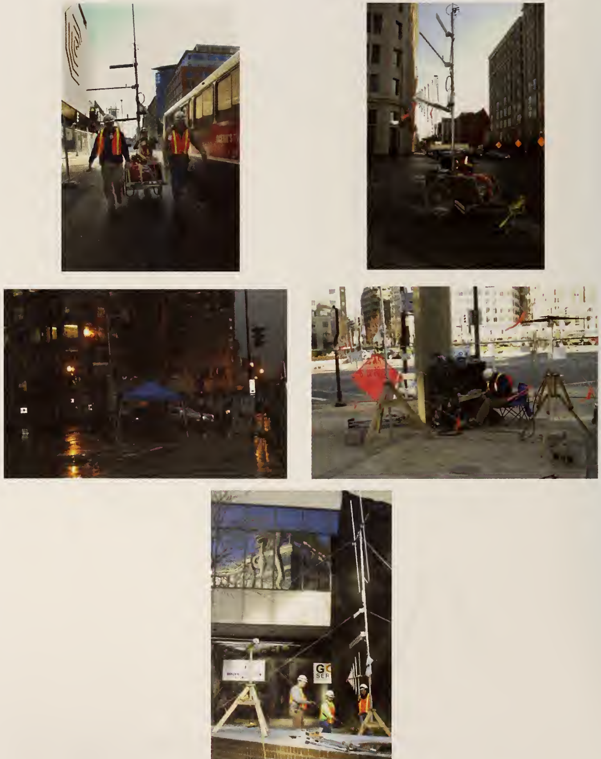
Figure 12. Photos of the antenna system mounted on a tripod and mounted to the mobile cart. The receiving instruments are protected inside the container near the tripod and inside the cart assembly when portable.
