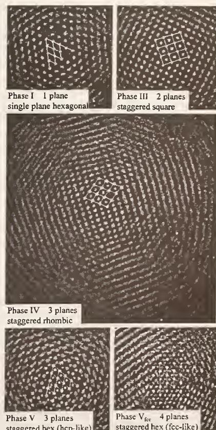
Fig. 2. Top-view (x, y) images of the five structural phases observed in the experiment, with lines showing a fit of the central ions to the indicated structure.
