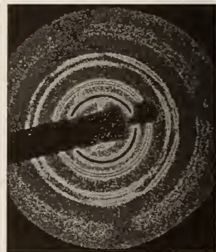
Fig. 2. Time-integrated Bragg diffraction pattern obtained with the CCD camera. Rotation of the plasma causes the diffraction spots to be smeared into circles. The long rectangular shadow is due to the laser beam deflector. The small circular shadow is due to the hole in the mirror. The four linear shadows forming a large square are due to a wire mesh. Here, \omega_r = 2\pi \times 128 kHz, n_0 = 3.90 \times 10^8 \text{ cm}^{-3} , N = 5 \times 10^5 , \alpha = 1.00 , and 2r_0 = 1.35 mm.
