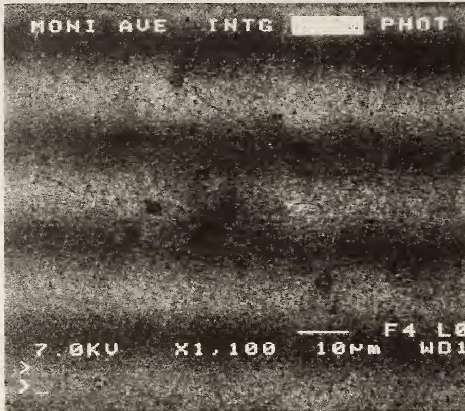
Figure 13. Typical moiré fringe field at 1100× obtained under ambient conditions.
