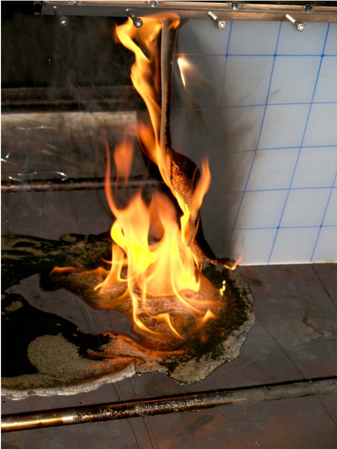
Figure 21. Pool-assisted fire growth on a vertical, 3 mm thick sheet of polypropylene.
