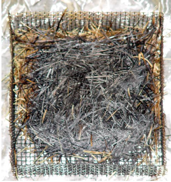
Figure 34. Bottom (left) and top (right) views of a May tall fescue fuel bed are shown after the fuel was removed from the heated plate held at 341 °C with no wind applied. Glowing combustion was observed after 235 s.
