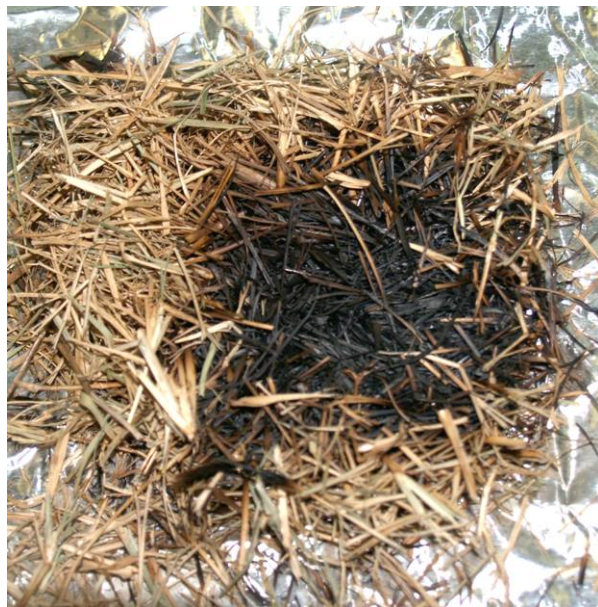
Figure 47. Bottom (left) and top (right) views of an August tall fescue fuel bed are shown after the fuel was removed from the heated plate held at 300 °C with no wind applied. No glowing combustion was observed.
