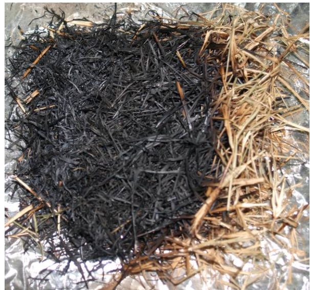
Figure 49. Bottom (left) and top (right) views of an August tall fescue fuel bed are shown after the fuel was removed from the heated plate held at 310 °C with a low wind applied. Glowing combustion and flaming were observed.
