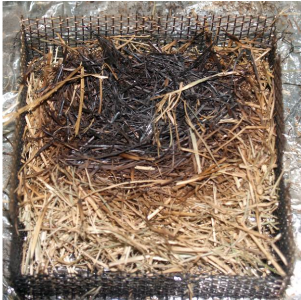
Figure 48. Bottom (left) and top (right) views of an August tall fescue fuel bed are shown after the fuel was removed from the heated plate held at 290 °C with no wind applied. No glowing combustion was observed.
