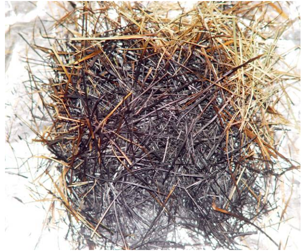
Figure 34. Bottom (left) and top (right) views of a May tall fescue fuel bed are shown after the fuel was removed from the heated plate held at 341 °C with no wind applied. Glowing combustion was observed after 235 s.
