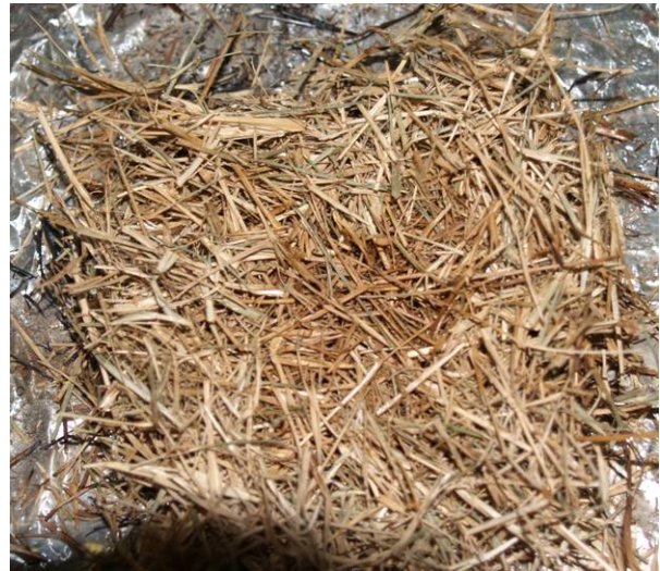
Figure 48. Bottom (left) and top (right) views of an August tall fescue fuel bed are shown after the fuel was removed from the heated plate held at 290 °C with no wind applied. No glowing combustion was observed.
