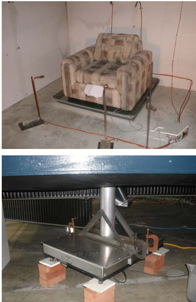
Figure 94. Example of mass loss measurement showing upholstered chair on load cell prior to one of the flaming ignition tests and load cell apparatus mounted beneath manufactured home
