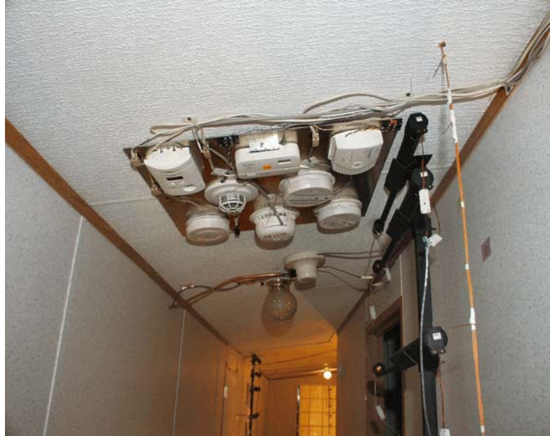
Figure 1. Sample sensor test board used during tests of residential smoke alarms
