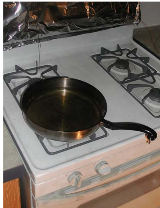
Figure 86. Heating ignition source with cooking oil
