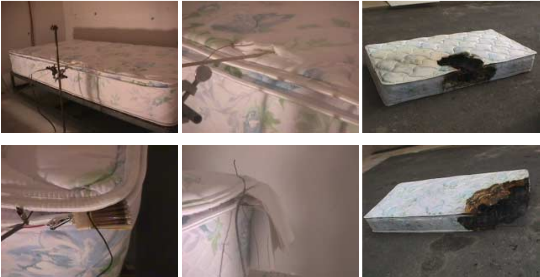
Figure 4. Twin-size mattresses before and after smoldering (1 st row) and flaming (2 nd row) fire tests
