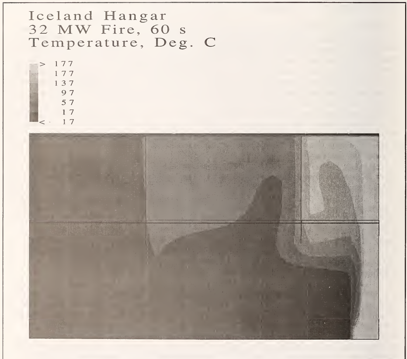
Figure 65. Side view of the 22 m high facility in a plane through the fire center. The draft curtains are represented by two vertical lines extending from the ceiling to just below the side roof level. The 32 MW fire is located on the hangar floor at the right side of the figure.
