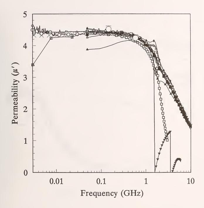
Figure 3a. Measured relative permeability,  $\mu_{r}$ ' for Material 3
