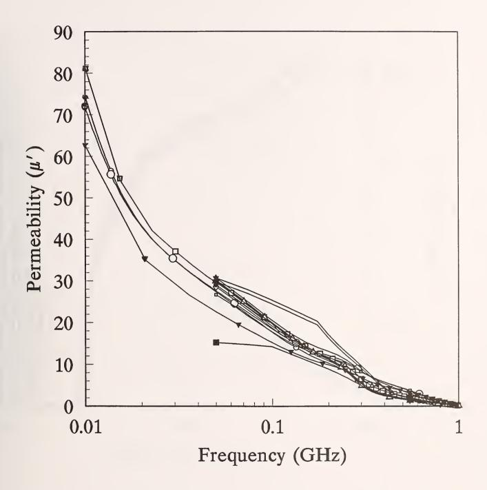
Figure 1a. Measured relative permeability,  $\mu_r$  for Material 1 (linear)
