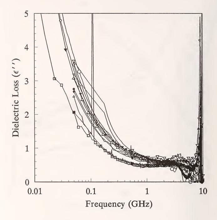
Figure 2f. Measured dielectric loss,  $\epsilon_r$ " for Material 2
