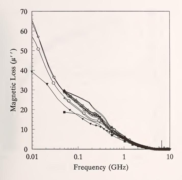
Figure 1c. Measured magnetic loss,  $\mu_r$ " for Material 1 (linear)
