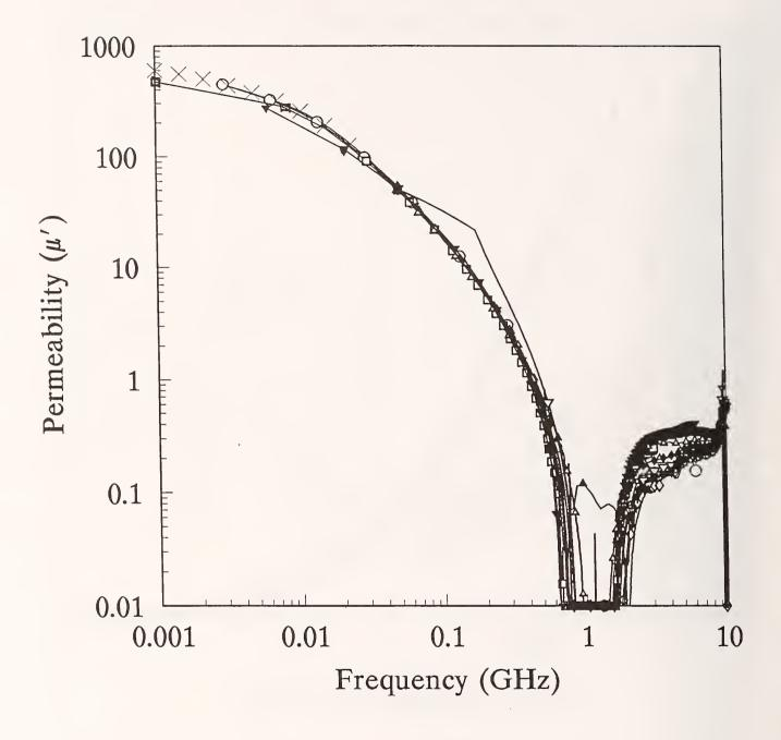
Figure 2b. Measured relative permeability,  $\mu_r$  for Material 2 (log)
