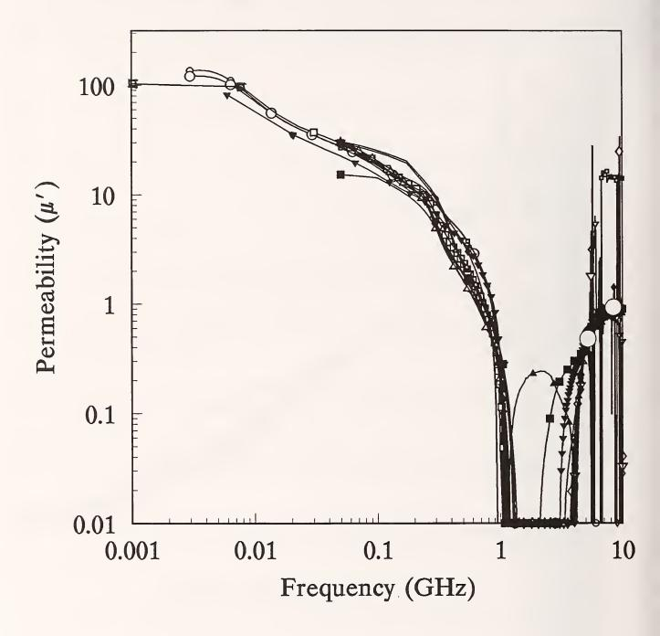
Figure 1b. Measured relative permeability,  $\mu_{r}$  for Material 1 (log)
