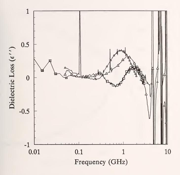
Figure 4f. Measured dielectric loss,  $\varepsilon_r$ " for Material 4
