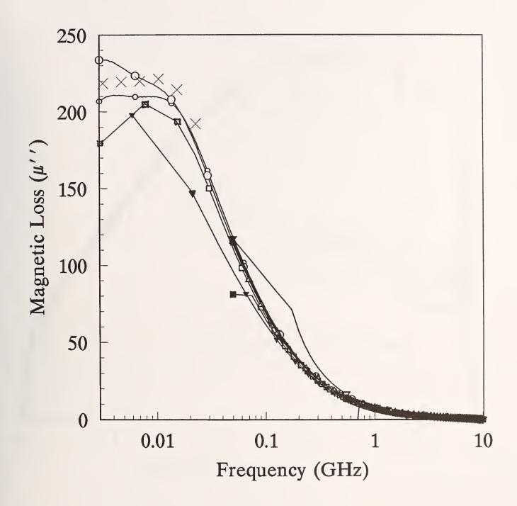
Figure 2c. Measured magnetic loss,  $\mu_r$ " for Material 2 (linear)
