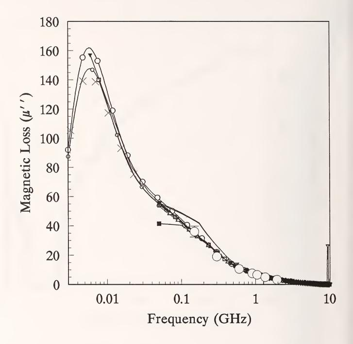
Figure 5c. Measured magnetic loss,  $\mu_r$ " for Material 5 (linear)
