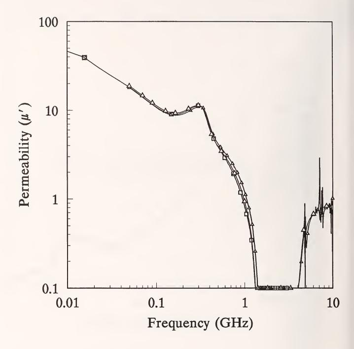
Figure 4b. Measured relative permeability,  $\mu_r$  for Material 4 (log)
