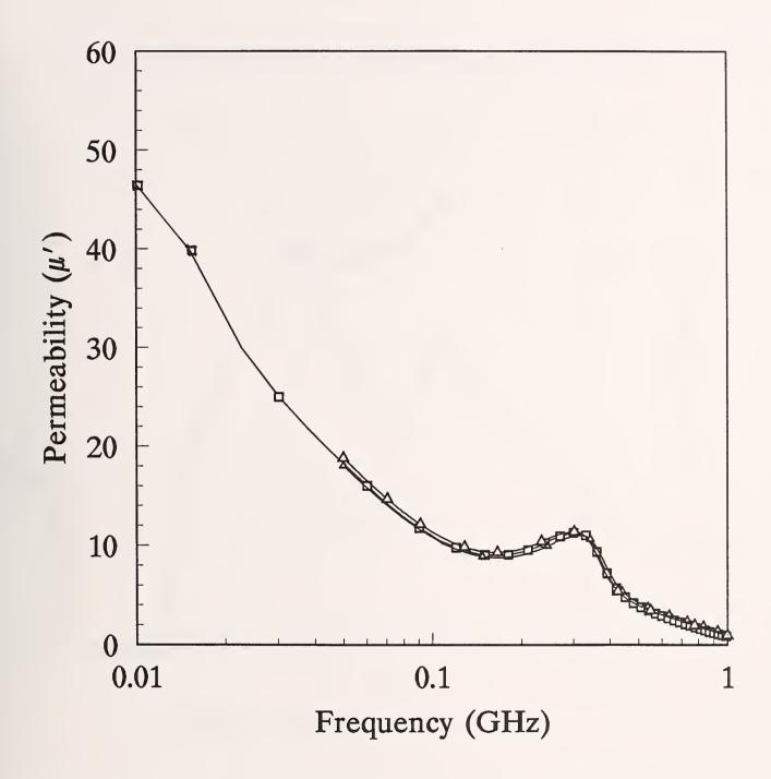
Figure 4a. Measured relative permeability,  $\mu_r$  for Material 4 (linear)
