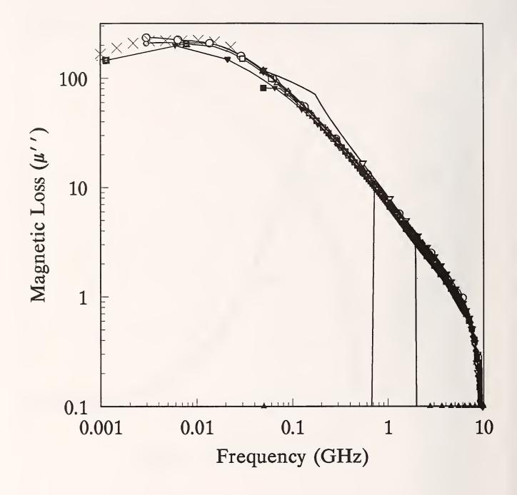
Figure 2d. Measured magnetic loss,  $\mu_r$ " for Material 2 (log)
