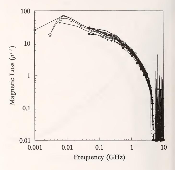
Figure 1d. Measured magnetic loss,  $\mu_r$ " for Material 1 (log)
