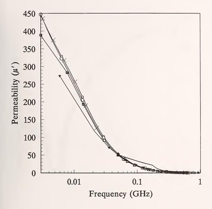
Figure 2a. Measured relative permeability,  $\mu_r$  for Material 2 (linear)
