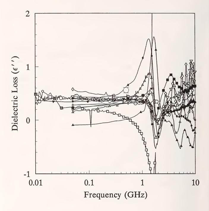
Figure 3f. Measured dielectric loss,  $\varepsilon_r$ " for Material 3
