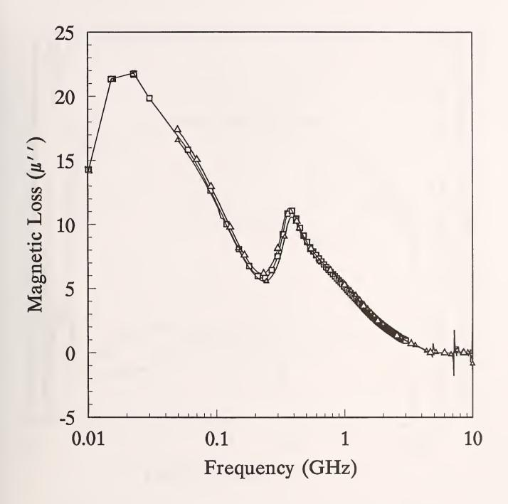
Figure 4c. Measured magnetic loss,  $\mu_r$ " for Material 4
