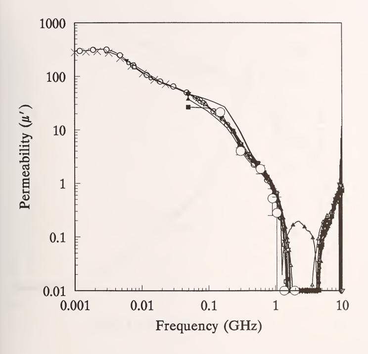
Figure 5b. Measured relative permeability,  $\mu_{r}^{\, \prime}$  for Material 5 (log)
