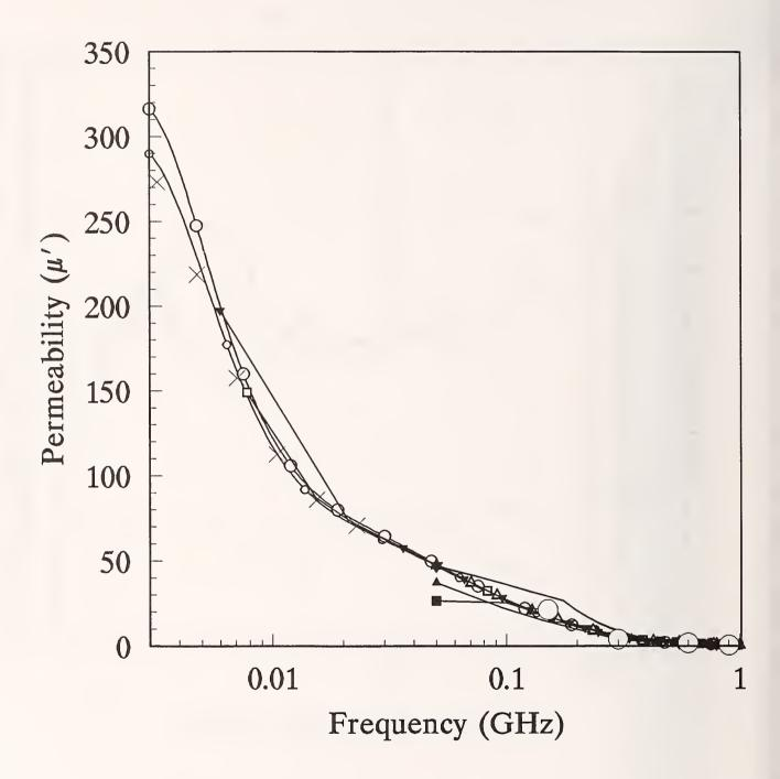
Figure 5a. Measured relative permeability,  $\mu_{r}$  for Material 5 (linear)
