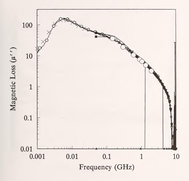
Figure 5d. Measured magnetic loss,  $\mu_r$ " for Material 5 (log)
