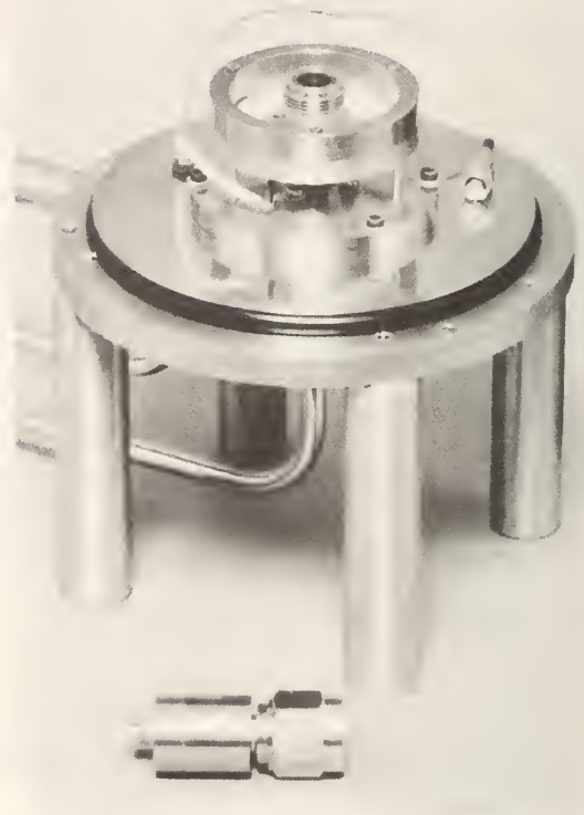
Figure 1.1 Coaxial microcalorimeter and coaxial reference standard.
