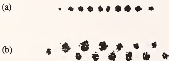
Fig. 3. Images taken of crystallized structures of ^{199}\text{Hg}^+ ions in a linear rf trap like the one of Fig. 2. In (a), 10 ions form into a string with length 220 \mu\text{m} . In (b), the the lowest energy configuration for 13 ions is a zig-zag structure. In (a) and (b), the trap conditions are different but the magnification is the same. (Ref. 13.)
