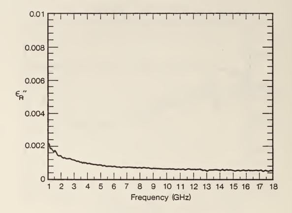
Figure 2.10  $\epsilon_R''$  of air in a coaxial line for empty air line using TR method. The worst case uncertainty at 10 GHz,  $\Delta \epsilon_R'' = 0.0012$ .
