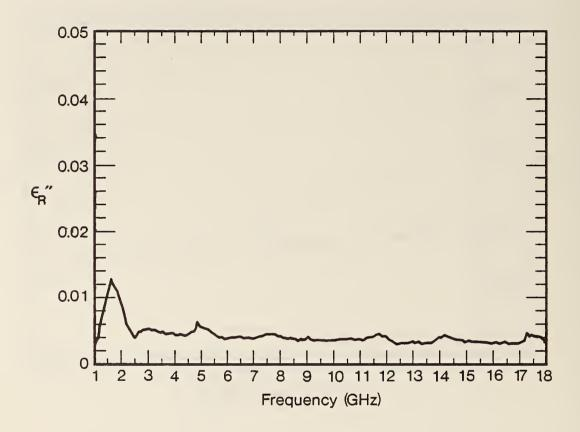
Figure 2.12 Calculated  $\epsilon_R''$  for PTFE in a coaxial line as function of frequency with TR method. The worst case uncertainty at 10 GHz,  $\Delta \epsilon_R'' = 0.0017$ .
