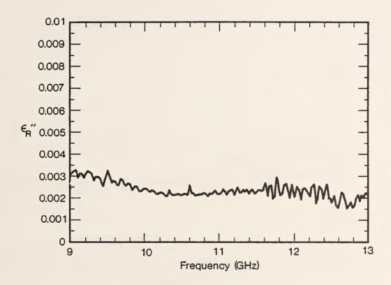
Figure 3.6  $\epsilon_R''$  using SCL in X-band waveguide for cross-linked polystyrene. The worst case uncertainty,  $\Delta \epsilon_R'' = 0.003$ , at 10 GHz.
