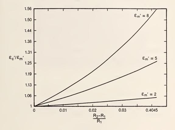
Figure 6.2 The gap correction calculated for various values of  $\epsilon'_R$ , where  $R_2, R_1$  are the radii of the inner conductor and sample respectively.
