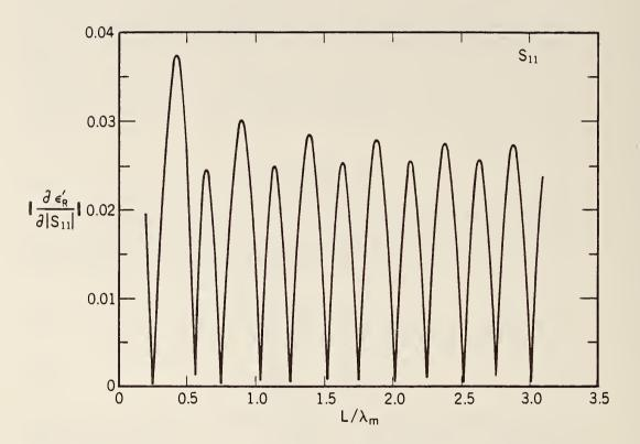
Figure 3.9 The derivative of  $\epsilon_R'$  with respect to  $|S_{11}|$  with  $\epsilon_R^* = (30.0, 0.01)$ .
