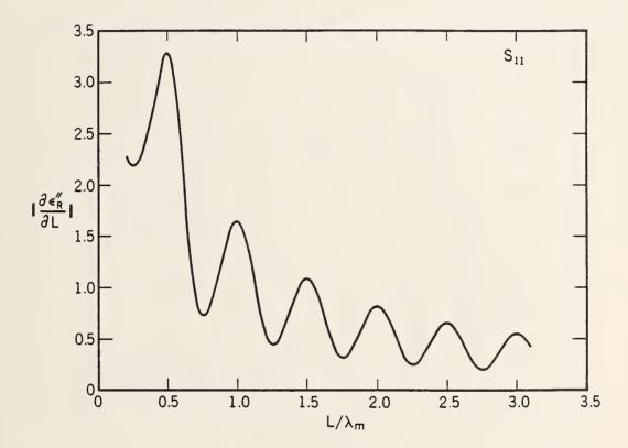
Figure 3.14 The derivative of  $\epsilon_R''$  with respect to length with  $\epsilon_R^* = (30.0, 0.01)$ .
