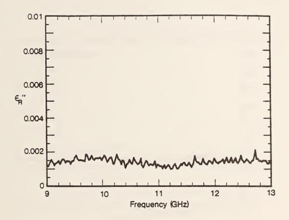
Figure 3.4  $\epsilon_R''$  using SCL in X-band waveguide for PTFE. The worst case uncertainty,  $\Delta \epsilon_R'' = 0.004$ , at 10 GHz.
