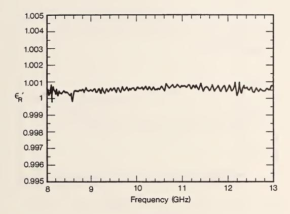
Figure 2.13  $\epsilon_R'$  of air in a X-band waveguide for empty air line using TR method. The worst case uncertainty at 10 GHz,  $\Delta\epsilon_R'=0.005$ .
