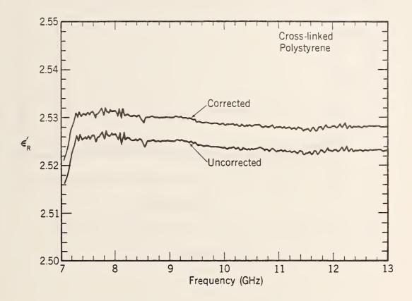
Figure 2.15 Calculated  $\epsilon_R'$  with and without gap correction for cross linked polystyrene in a X-band waveguide as function of frequency with TR method. The worst case uncertainty at 10 GHz,  $\Delta \epsilon_R' = 0.011$ .
