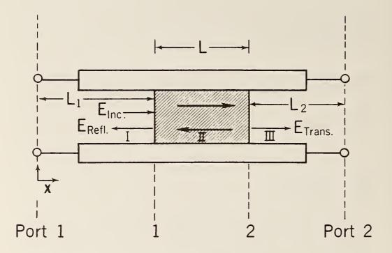
Figure 2.1: A dielectric sample in a transmission line and the incident(inc) and reflected (refl) electric field distributions in the regions I, II, and III. Port 1 and port 2 denote calibration reference plane positions.
