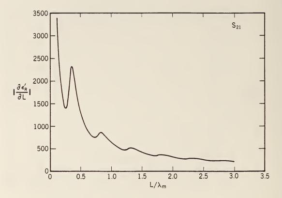
Figure 2.25 The derivative of  $\epsilon_R'$  with respect to length using  $S_{21}$  with  $\epsilon_R^* = (10.0, 0.01)$ .
