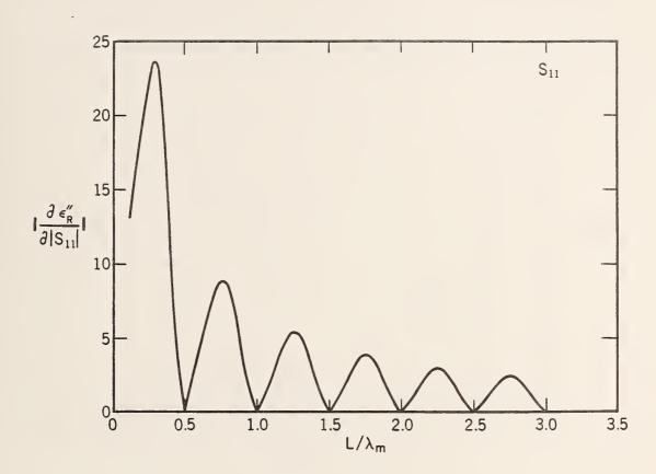
Figure 2.28 The derivative of  $\epsilon_R''$  with respect to  $|S_{11}|$  with  $\epsilon_R^* = (5.0, 0.01)$ .
