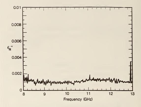
Figure 2.16 Calculated  $\epsilon_R''$  with and without gap correction for cross-linked polystyrene in a X-band waveguide as function of frequency with TR method. The worst case uncertainty at 10 GHz,  $\Delta \epsilon_R'' = 0.002$ .
