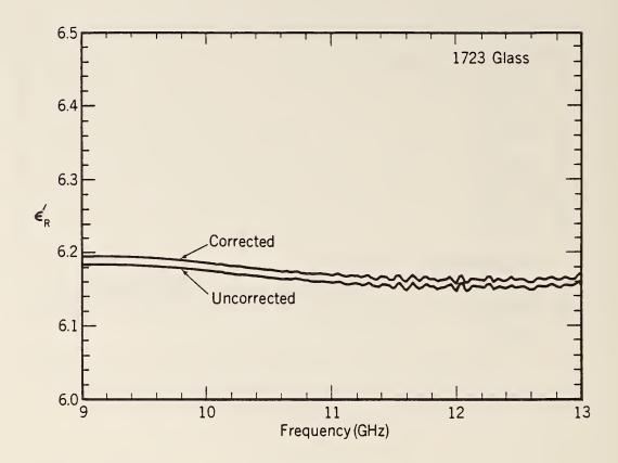
Figure 3.7  $\epsilon_R'$  with and without gap correction using SCL for 1723 glass. The worst case uncertainty,  $\Delta \epsilon_R' = 0.021$ , at 10 GHz.
