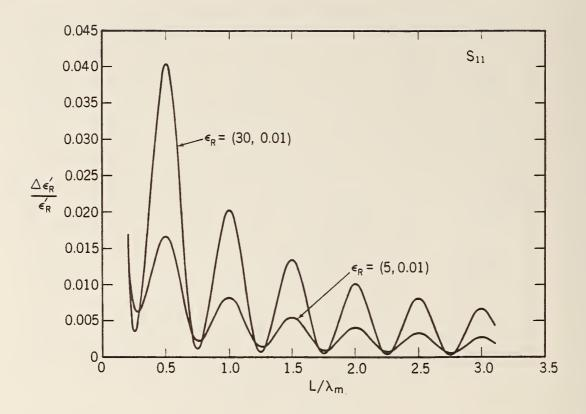
Figure 3.15 The relative uncertainty in  $\epsilon_R'$  for  $S_{11}$  using SCL for a low-loss material, with  $\epsilon_R^* = (5.0,0.01)$  and (30.0,0.01).
