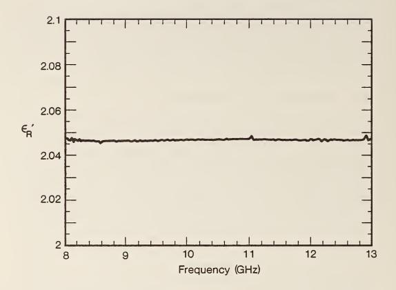
Figure 3.3  $\epsilon_R'$  using SCL in X-band waveguide for PTFE. The worst case uncertainty,  $\Delta \epsilon_R' = 0.011$ , at 10 GHz.
