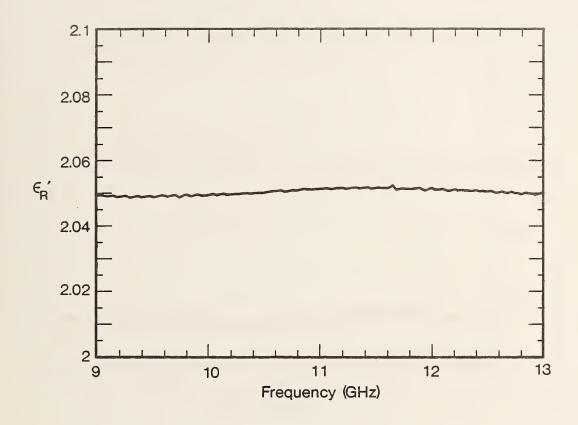
Figure 2.17 Calculated  $\epsilon_R'$  for PTFE in waveguide as function of frequency with TR method. The worst case uncertainty at 10 GHz,  $\Delta\epsilon_R' = 0.009$ .
