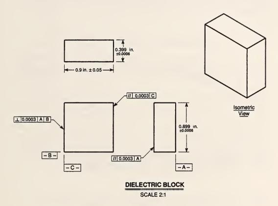
Figure 2.6 Sample specifications for a rectangular sample in inches.
