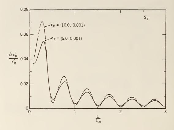
Figure 2.34 The relative uncertainty in  $\epsilon_R(\omega)$  for  $S_{11}$  for a low-loss material as a function of normalized length, with  $\epsilon_R^* = (5.0, 0.001)$  in solid line and (10.0, 0.001) in dashed line.
