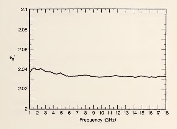
Figure 2.11 Calculated  $\epsilon_R'$  for PTFE in a coaxial line as function of frequency with TR method. The worst case uncertainty at 10 GHz,  $\Delta\epsilon_R' = 0.009$ .
