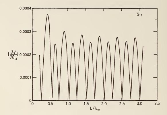
Figure 3.11 The derivative of  $\epsilon_R'$  with respect to  $\theta$  with  $\epsilon_R^* = (30.0, 0.01)$ .
