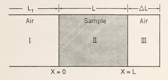
Figure 3.1 A transmission line with a short-circuit termination.
