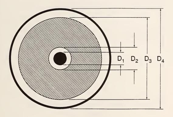
Figure 6.1 A coaxial sample in holder with air gaps near conductors.
