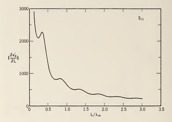
Figure 2.31 The derivative of  $\epsilon_R'$  with respect to length using  $S_{11}$  with  $\epsilon_R^* = (5.0, 0.01)$ .
