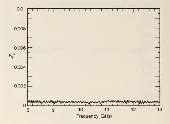
Figure 2.14  $\epsilon_R''$  of air in a X-band waveguide for empty air line using TR method. The worst case uncertainty at 10 GHz,  $\Delta\epsilon_R''=0.0012$ .
