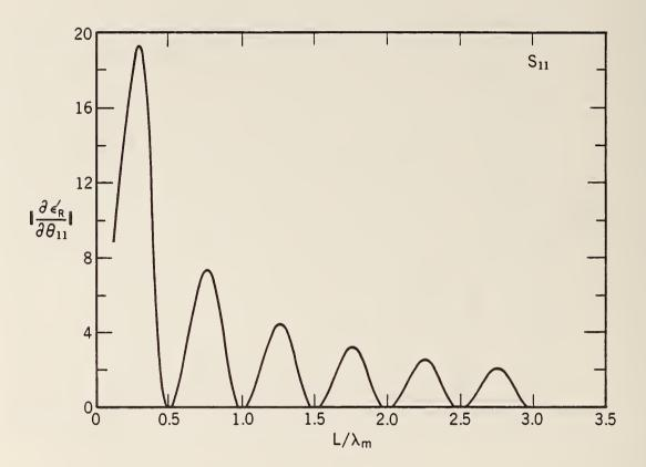
Figure 2.29 The derivative of  $\epsilon_R'$  with respect to  $\theta$  using  $S_{11}$  with  $\epsilon_R^* = (5.0, 0.01)$ .
