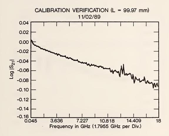
Figure 2.7 System diagnostic example for  $|S_{21}|$ .
