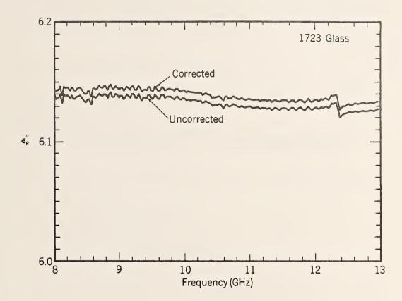
Figure 2.19  $\epsilon_R'$  with and without gap correction using TR method for 1723 glass in a X-band waveguide. The worst case uncertainty at 10 GHz,  $\Delta \epsilon_R' = 0.013$ .
