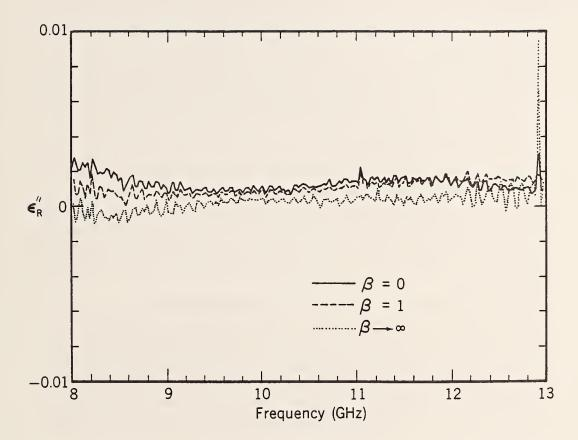
Figure 2.4 The imaginary part of the permittivity obtained from eq (2.38) for various values of  $\beta$ . The dotted line is for  $\beta \to \infty$ , the solid line for  $\beta = 0$  and the dashed line for  $\beta = 1$ .
