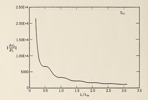
Figure 3.13 The derivative of  $\epsilon_R'$  with respect to length with  $\epsilon_R^* = (30.0, 0.01)$ .
