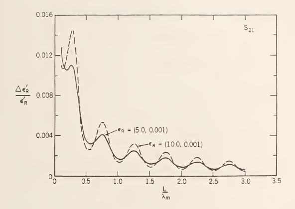
Figure 2.33 The relative uncertainty in  $\epsilon_R(\omega)$  for  $S_{21}$  for a low-loss material as a function of normalized length, with  $\epsilon_R^* = (5.0, 0.001)$  in solid line and (10.0,0.001) in dashed line.
