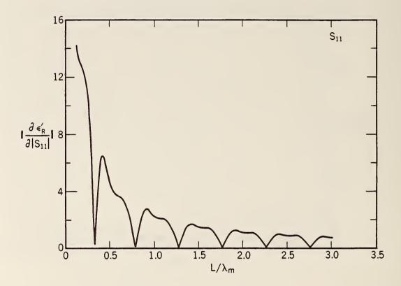
Figure 2.27 The derivative of  $\epsilon_R'$  with respect to  $|S_{11}|$  with  $\epsilon_R^* = (5.0, 0.01)$ .
