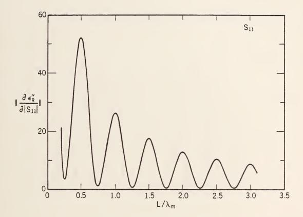
Figure 3.10 The derivative of  $\epsilon_R''$  with respect to  $|S_{11}|$  with  $\epsilon_R^* = (30.0, 0.01)$ .
