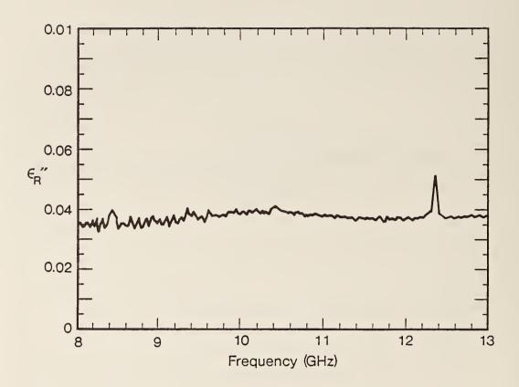
Figure 2.20  $\epsilon_R''$  using TR method for 1723 glass in a X-band waveguide. The worst case uncertainty at 10 GHz,  $\Delta \epsilon_R'' = 0.009$ .
