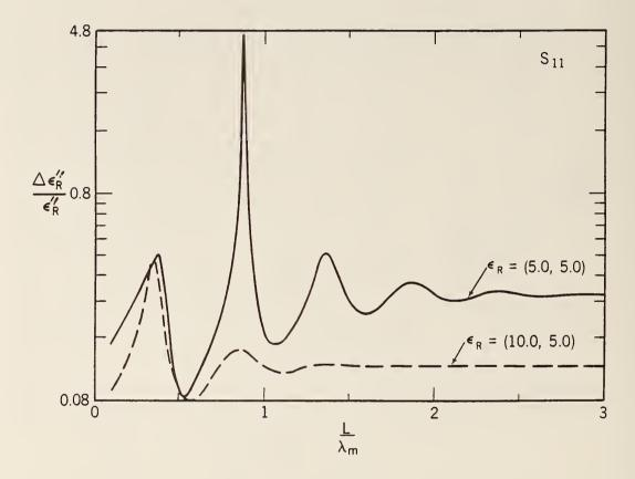
Figure 2.38 The relative uncertainty in  $\epsilon_R''(\omega)$  for  $S_{11}$  for a high-loss material as a function of normalized length with  $\epsilon_R^* = (5.0, 5.0)$  in solid line and (10.0, 5.0) in dashed line.
