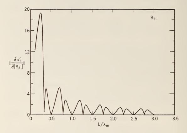
Figure 2.21 The derivative of  $\epsilon_R'$  with respect to  $|S_{21}|$  with  $\epsilon_R^* = (10.0, 0.01)$ .
