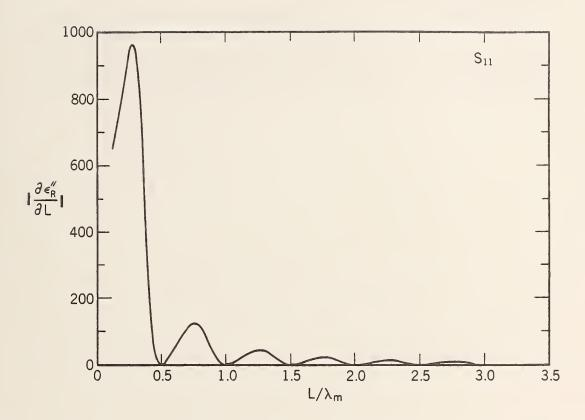
Figure 2.32 The derivative of  $\epsilon_R''$  with respect to length using  $S_{11}$  with  $\epsilon_R^* = (5.0, 0.01)$ .
