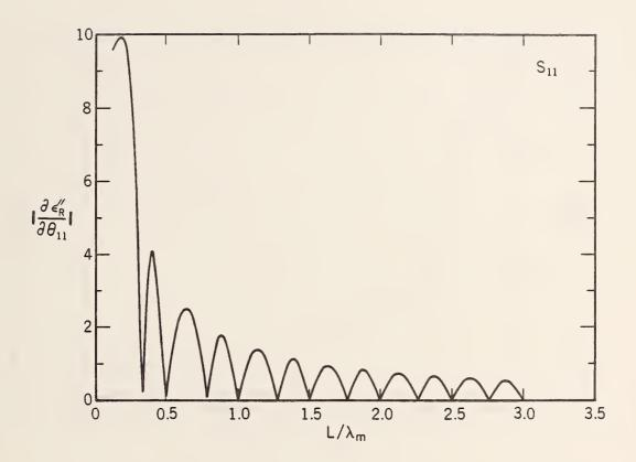
Figure 2.30 The derivative of  $\epsilon_R''$  with respect to  $\theta$  using  $S_{11}$  with  $\epsilon_R^* = (5.0, 0.01)$ .
