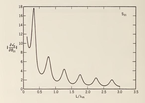
Figure 2.23 The derivative of  $\epsilon_R'$  with respect to  $\theta$  using  $S_{21}$  with  $\epsilon_R^* = (10.0, 0.01)$ .
