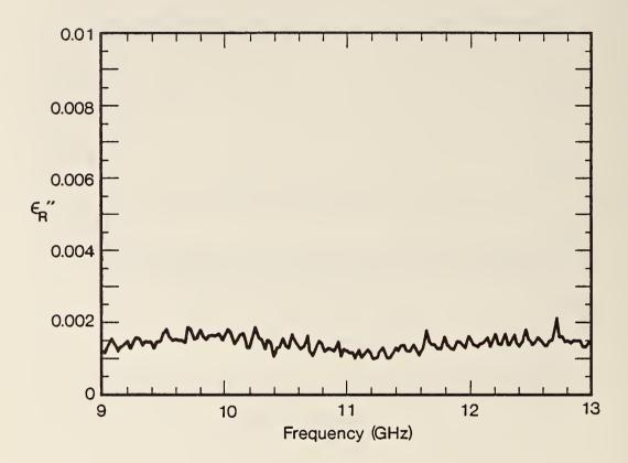
Figure 2.18 Calculated  $\epsilon_R''$  for PTFE in waveguide as function of frequency with TR method. The worst case uncertainty at 10 GHz,  $\Delta \epsilon_R'' = 0.0016$ .
