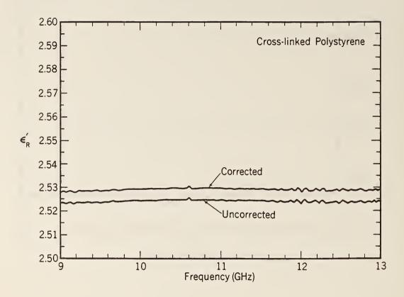
Figure 3.5  $\epsilon_R'$  with and without gap correction using SCL in X-band waveguide for cross-linked polystyrene. The worst case uncertainty,  $\Delta \epsilon_R' = 0.009$ , at 10 GHz.
