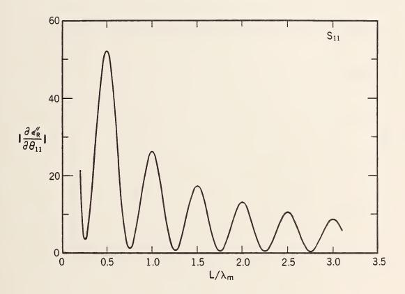
Figure 3.12 The derivative of  $\epsilon_R''$  with respect to  $\theta$  with  $\epsilon_R^* = (30.0, 0.01)$ .
