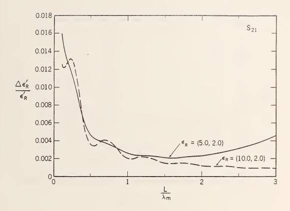
Figure 2.35 The relative uncertainty in  $\epsilon_R'(\omega)$  for  $S_{21}$  for a high-loss material as a function of normalized length, with  $\epsilon_R^* = (5.0, 2.0)$  in solid line and (10.0, 2.0) in dashed line.
