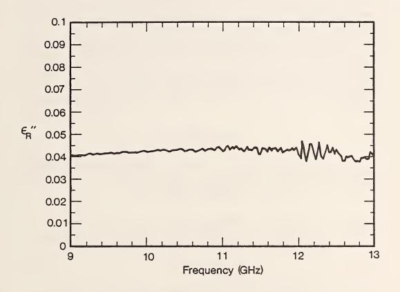
Figure 3.8  $\epsilon_R''$  with and without gap correction using SCL for 1723 glass. The worst case uncertainty,  $\Delta \epsilon_R'' = 0.009$ , at 10 GHz.
