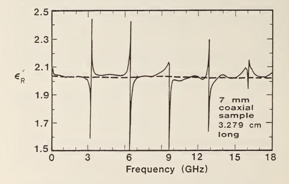
Figure 2.2: The determination of the permittivity of a polytetrafluoroethylene sample as a function of frequency using the Nicolson and Ross equations (solid line) and the iteration procedure (dashed line).
