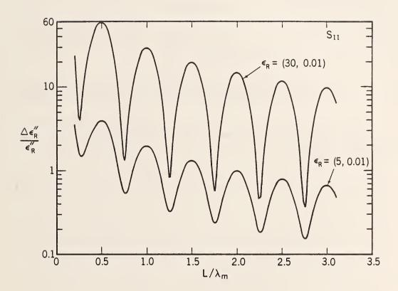
Figure 3.16 The relative uncertainty in  $\epsilon_R''$  for  $S_{11}$  for a low-loss material, with  $\epsilon_R^* = (5.0,0.01)$  and (30.0,0.01).
