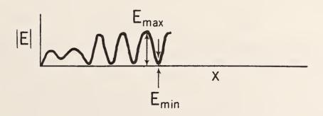
Figure 3.2 A transmission line containing sample with a slotted line measuring device for VSWR.
