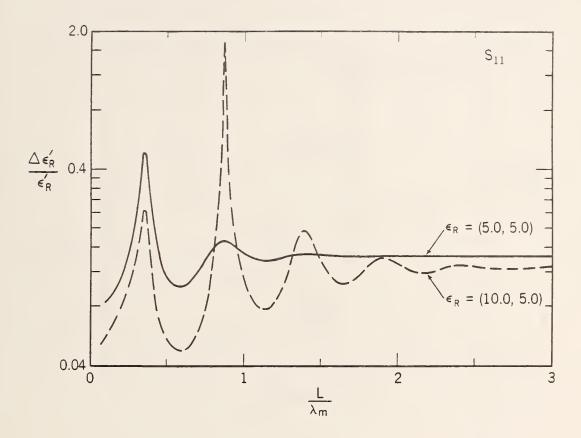
Figure 2.37 The relative uncertainty in  $\epsilon_R'(\omega)$  for  $S_{11}$  as a function of frequency for a high-loss material as a function of normalized length with  $\epsilon_R^* = (5.0, 5.0)$  in solid line and (10.0, 5.0) in dashed line.
