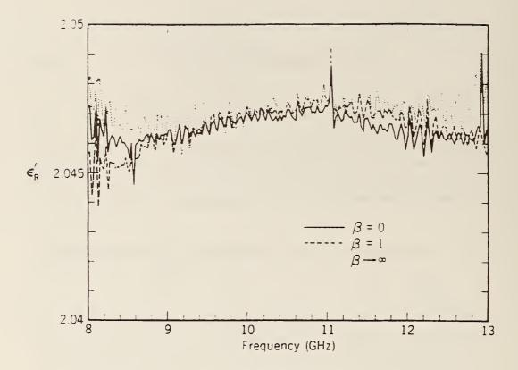
Figure 2.3 The real part of the permittivity obtained from eq (2.38) for various values of  $\beta$ . The dotted line is for  $\beta \to \infty$ , the solid line for  $\beta = 0$  and the dashed line for  $\beta = 1$ .
