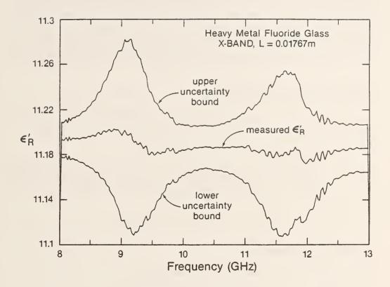
Figure 2.39 A plot of  $\epsilon_R'(\omega)$  from measurements on a heavy metal fluoride glass and uncertainty bounds.
