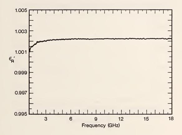
Figure 2.9  $\epsilon_R'$  of air in a coaxial line for empty air line using TR method. The worst case uncertainty at 10 GHz,  $\Delta \epsilon_R' = 0.005$ .
