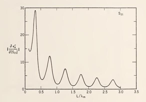
Figure 2.22 The derivative of  $\epsilon_R''$  with respect to  $|S_{21}|$  with  $\epsilon_R^* = (10.0, 0.01)$ .
