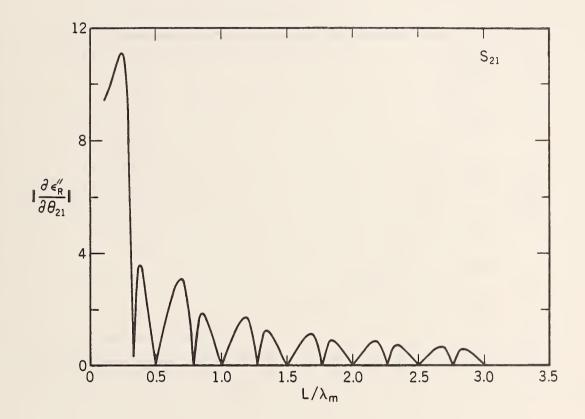
Figure 2.24 The derivative of  $\epsilon_R''$  with respect to  $\theta$  using  $S_{21}$  with  $\epsilon_R^* = (10.0, 0.01)$ .
