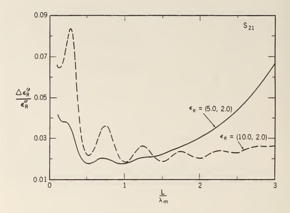
Figure 2.36 The relative uncertainty in  $\epsilon_R''(\omega)$  for  $S_{21}$  for a high-loss material as a function of normalized length, for  $\epsilon_R^* = (5.0, 2.0)$  in solid line and (10.0, 2.0) in dashed line.
