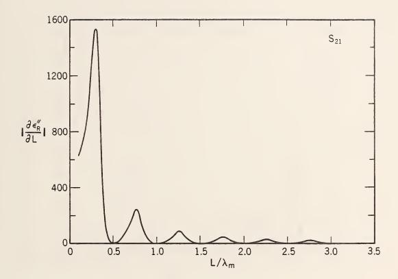
Figure 2.26 The derivative of  $\epsilon_R''$  with respect to length using  $S_{21}$  with  $\epsilon_R^* = (10.0, 0.01)$ .
