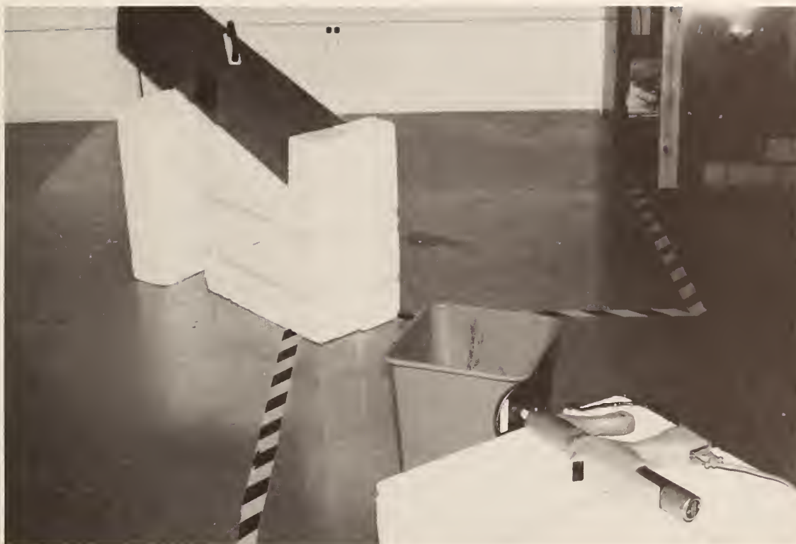
Figure 30. Measurement configuration for radiation by a metal trash can on a ground plane.
