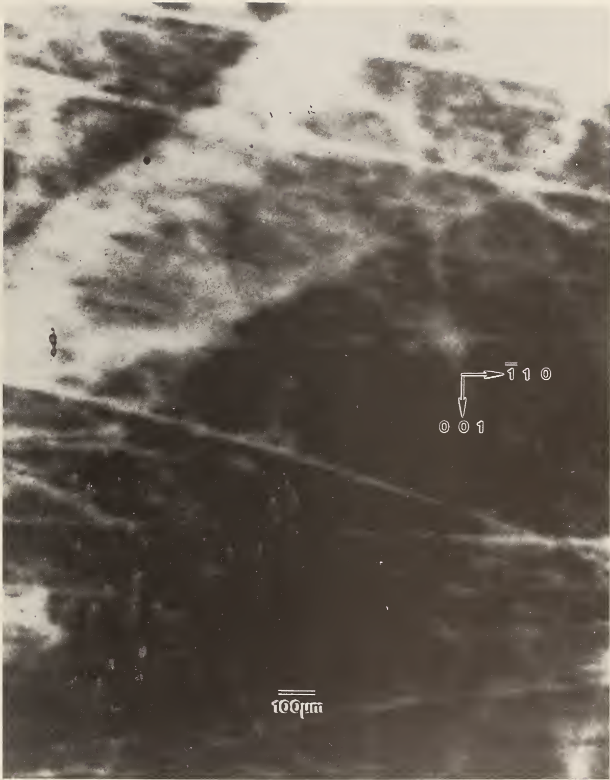
Figure 52. Enlargement of upper right portion of figure 40, (220) diffraction. Darker areas diffract more strongly.
