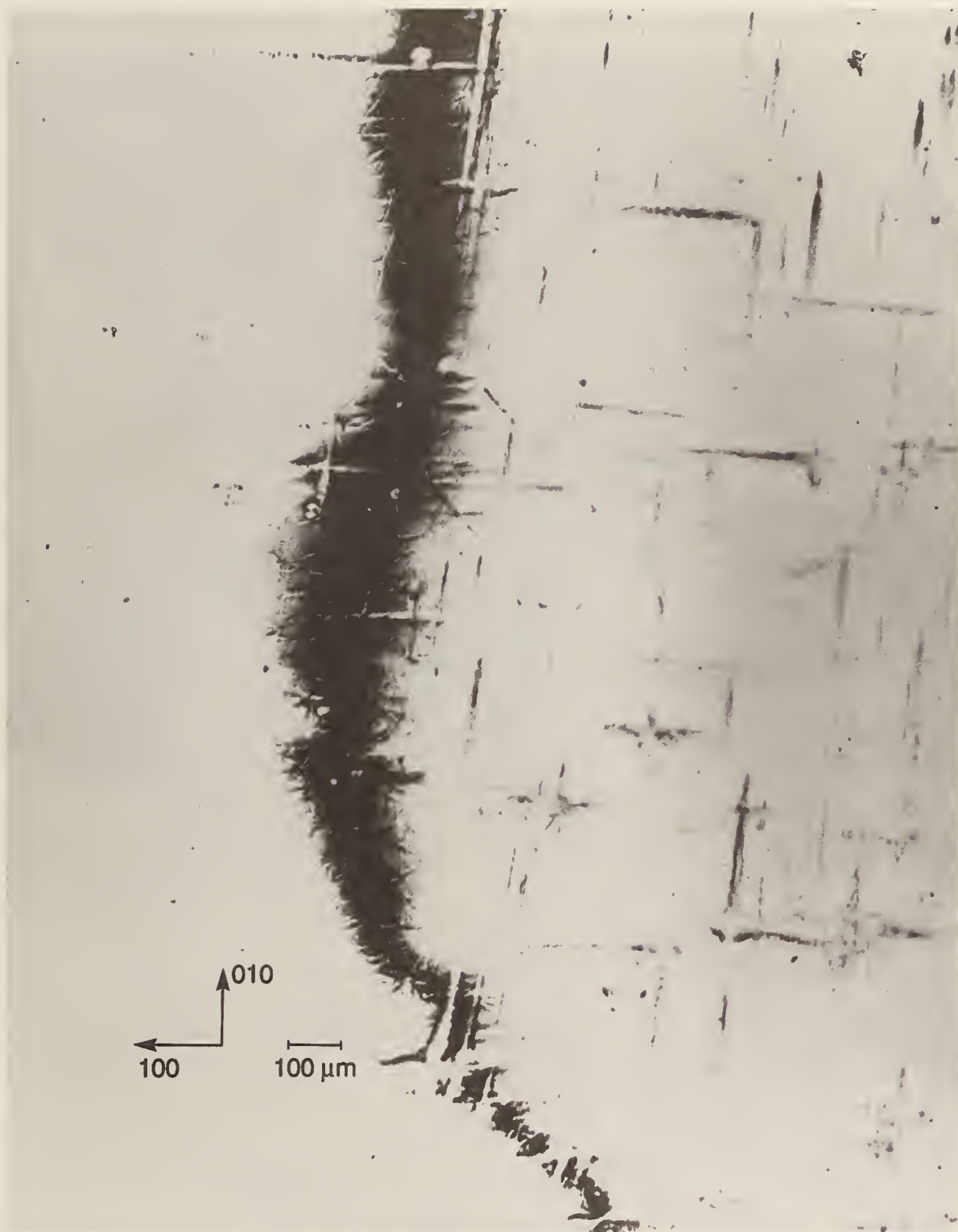
Figure 16. Enlargement of upper central portion of figure 3, (0 1 10) diffraction. The crystal region in this image is contiguous to the region imaged in (1 1 12) diffraction, figure 9, and in (1 1 10) diffraction, figure 12. Darker areas diffract more strongly.
