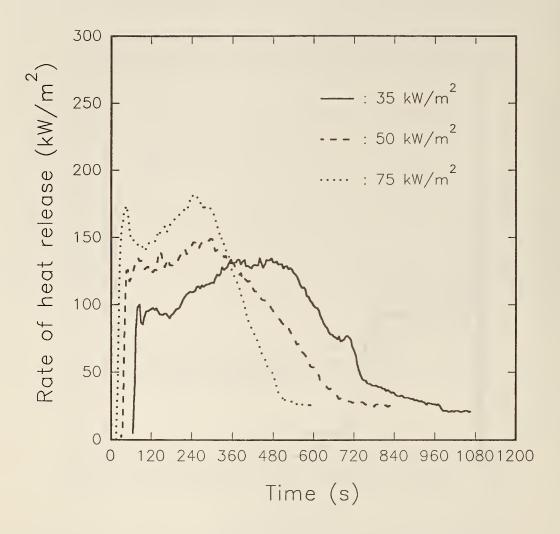
Figure 14. Heat release rates measured in the Cone Calorimeter for PVC
