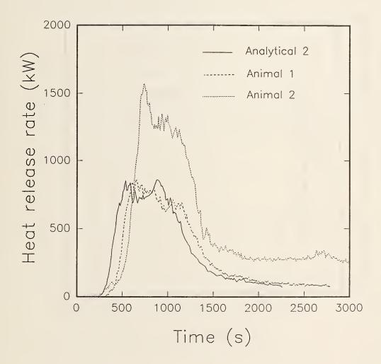
Figure 16. Heat release rates measured for DF in the real-scale tests
