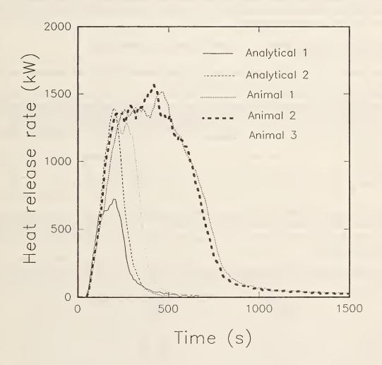
Figure 18. Heat release rates measured for PVC in the real-scale tests
