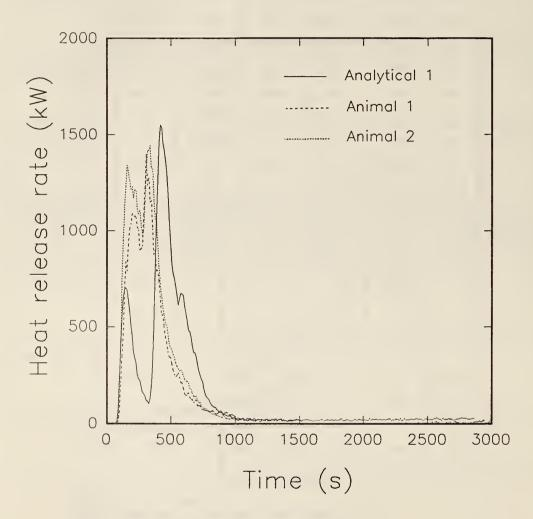
Figure 17. Heat release rates measured for RPU in the real-scale tests
