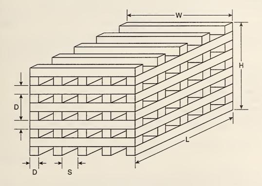
Figure 8. Construction of the test cribs
