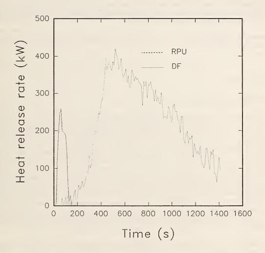
Figure 15. Heat release rates measured in the Furniture Calorimeter for cribs
