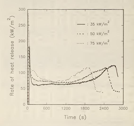
Figure 12. Heat release rates measured in the Cone Calorimeter for DF
