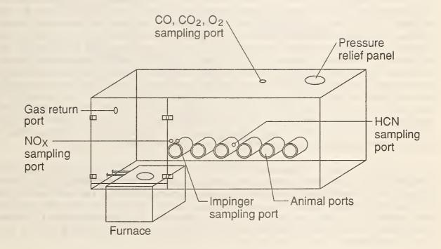
Figure 1. General view of the NBS Cup Furnace method
