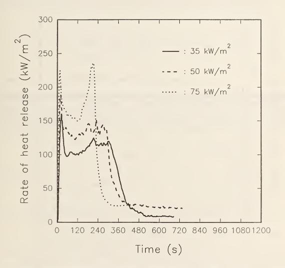
Figure 13. Heat release rates measured in the Cone Calorimeter for RPU
