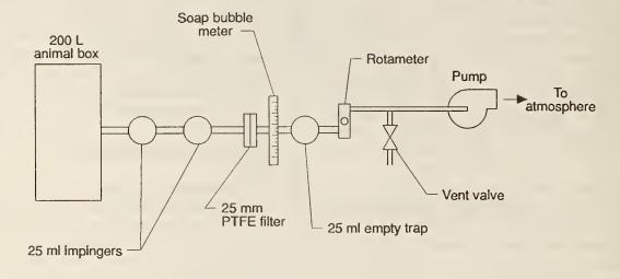
Figure 3. Impinger gas sampling in the NBS Cup Furnace method
