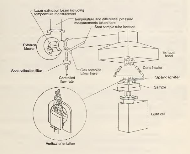
Figure 6. General view of the Cone Calorimeter
