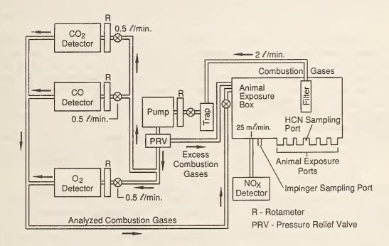
Figure 2. Gas sampling arrangements in the NBS Cup Furnace method
