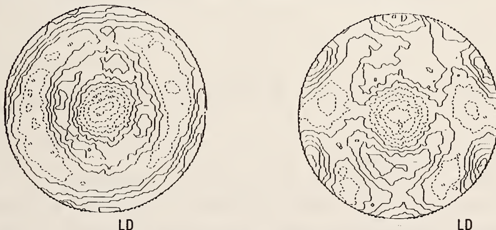
Figure 2. The 101 pole figures of the Ti samples S, P, and E. The center of each pole figure corresponds to the normal direction to the sample surface. The symbol LD in the pole figures of sample E indicates the longitudinal direction of the sample hemisphere, and in sample P it indicates the direction of the long diagonal of the rhombic shape. The densities lower than random intensity are shown by dotted contours, the lowest solid contour lines corresponding to "random." The contour intervals, in 0.1 m.r.d. units, are shown by the symbol ZSTEP in each pole figure.
