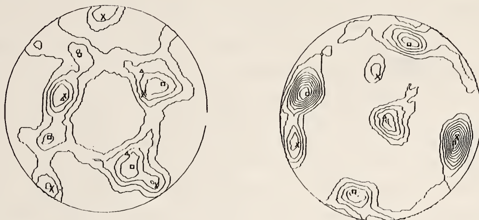
Figure 1. The 220 and 222 pole figures of the Ta sheet. The center of the pole figures correspond to the normal direction ( \chi = 90^\circ ) and the periphery to \chi = 20^\circ . The calculated pole density peak positions based on the three preferential slips were indicated with, squares for 100 slip plane, triangles for the 111 slip plane and x's for the 113 slip plane model. The contour levels of 1 m.r.d. or higher are given in steps of 0.5 m.r.d.
