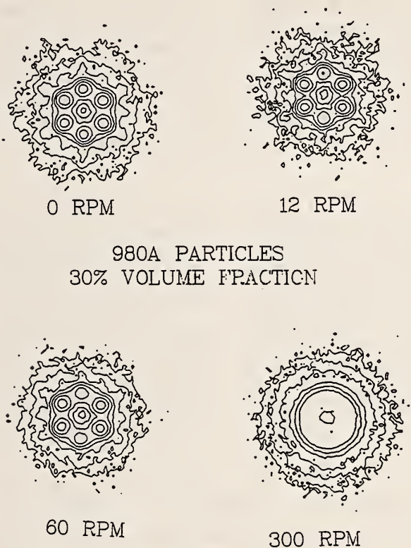
Figure 1. Change in the neutron scattered intensity pattern for a sheared colloidal suspension as a function of shear-rate. Note the shear induced melting to a liquid structure.
