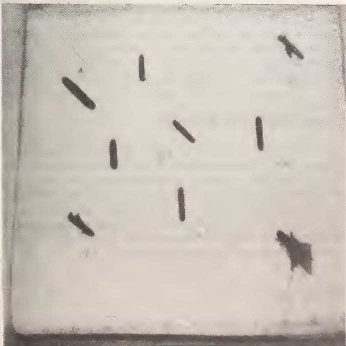
Figure 3-3. Sites for Various Cigarette Types Marked on a Damask Cushion, With Burn Scars Near the Marks. There were no Ignitions in these Tests
